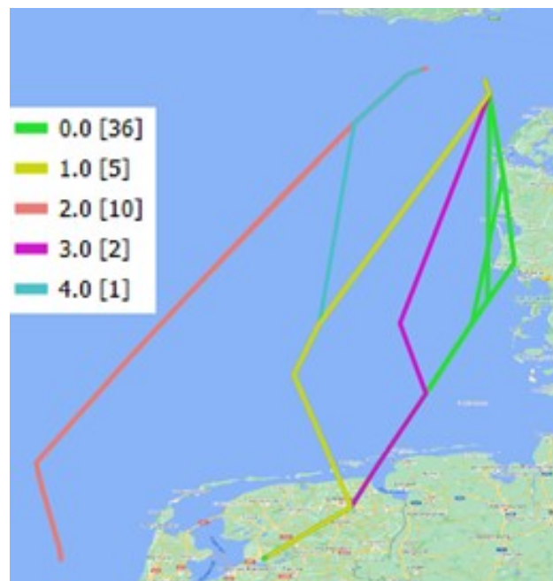
Figure 6: ENCN-EHAM OD pair routes for AIRAC 1813. The number of times the route has been used is indicated in brackets.
