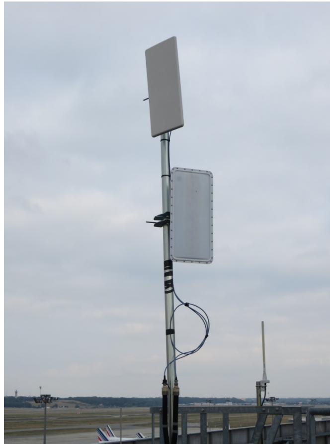
Figure 62: BS antennas vertical implementation
