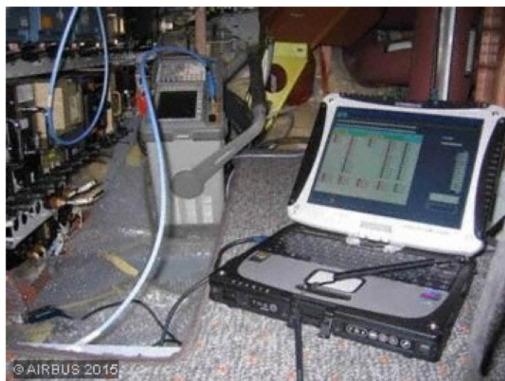
Figure 141: Aircraft tests – EMI - Spectrum Analyzer and PC (example)
