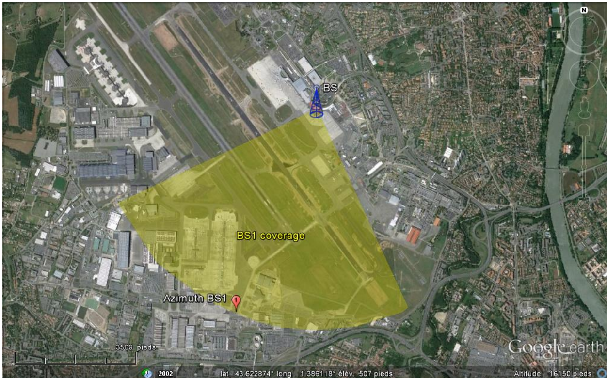
Figure 64: Laboratory Test - Theoretical BS1 coverage (Ratio 32:15)
