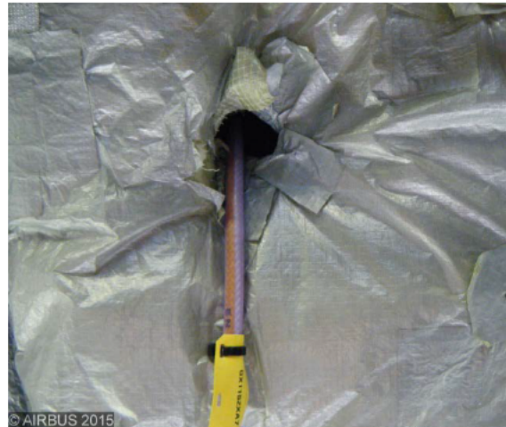
Figure 142: Aircraft tests – T207 – RF cable passing through fuselage to antenna
