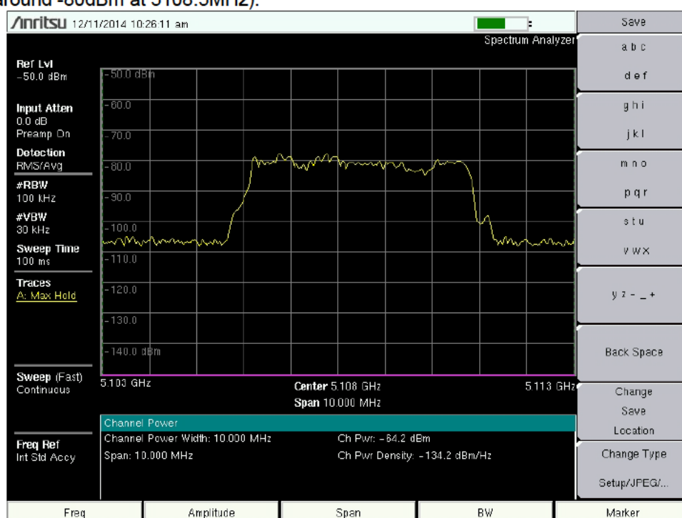
Figure 149: Aircraft tests – LOS Static test point at compensation area (5108.5MHz)
