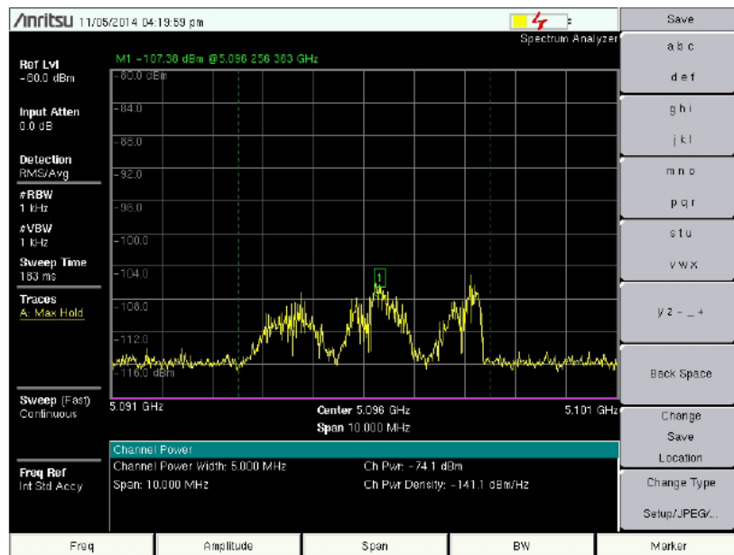
Figure 69: AeroMACS Bandwidth measure at 5096MHz
