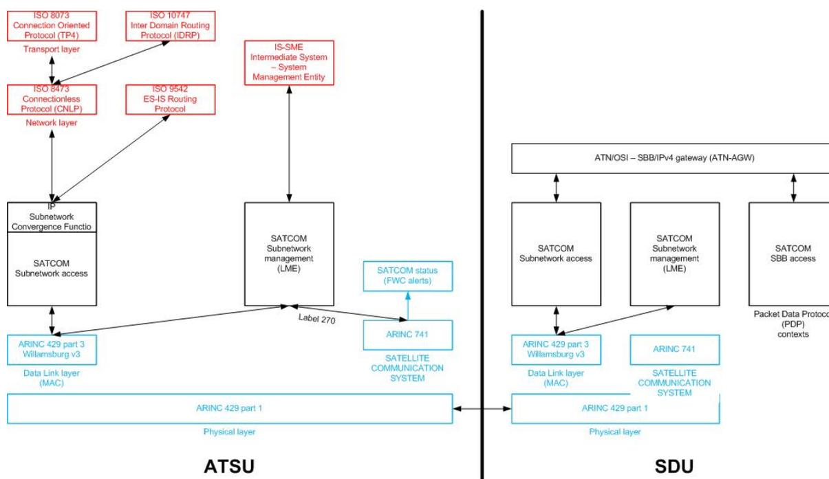
**Figure 3: Iris Precursor system Functional block Identification for airborne subsystem**
