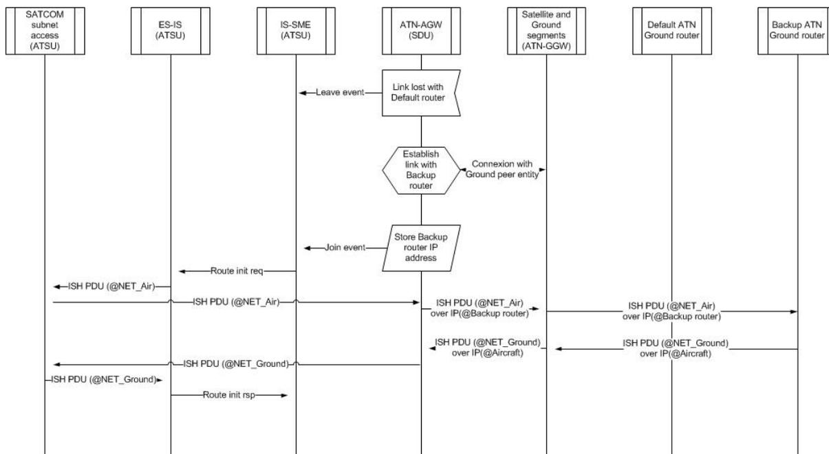
Figure 6: “ATN leave/join” sequence diagram (handover to backup AGR)
