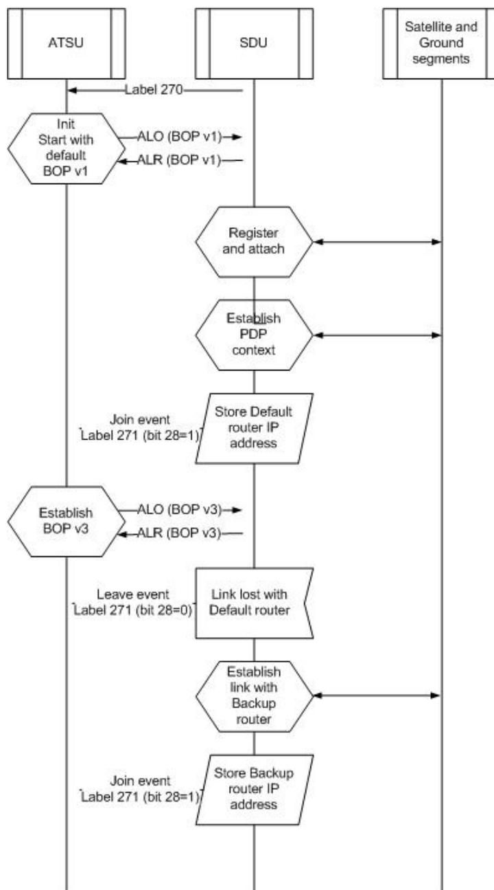
**Figure 7: Typical “P15.2.5 Iris Precursor” sequence diagram (Williamsburg protocol)**
