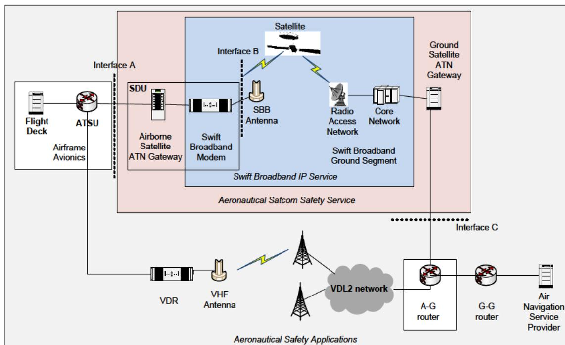
**Figure 1: End-End System Architectural Concept**
