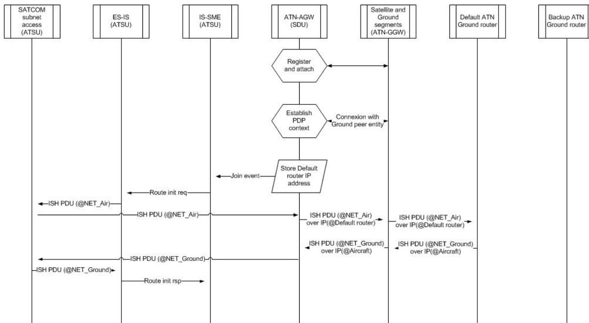
Figure 5: “ATN join” sequence diagram (with default AGR)
