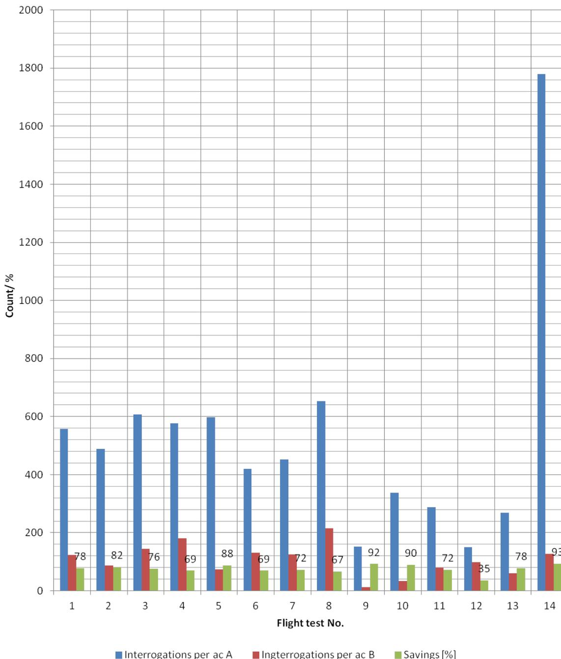
**Figure 31: Average number of all interrogations per aircraft for samples A and B and the savings (labelled).**
