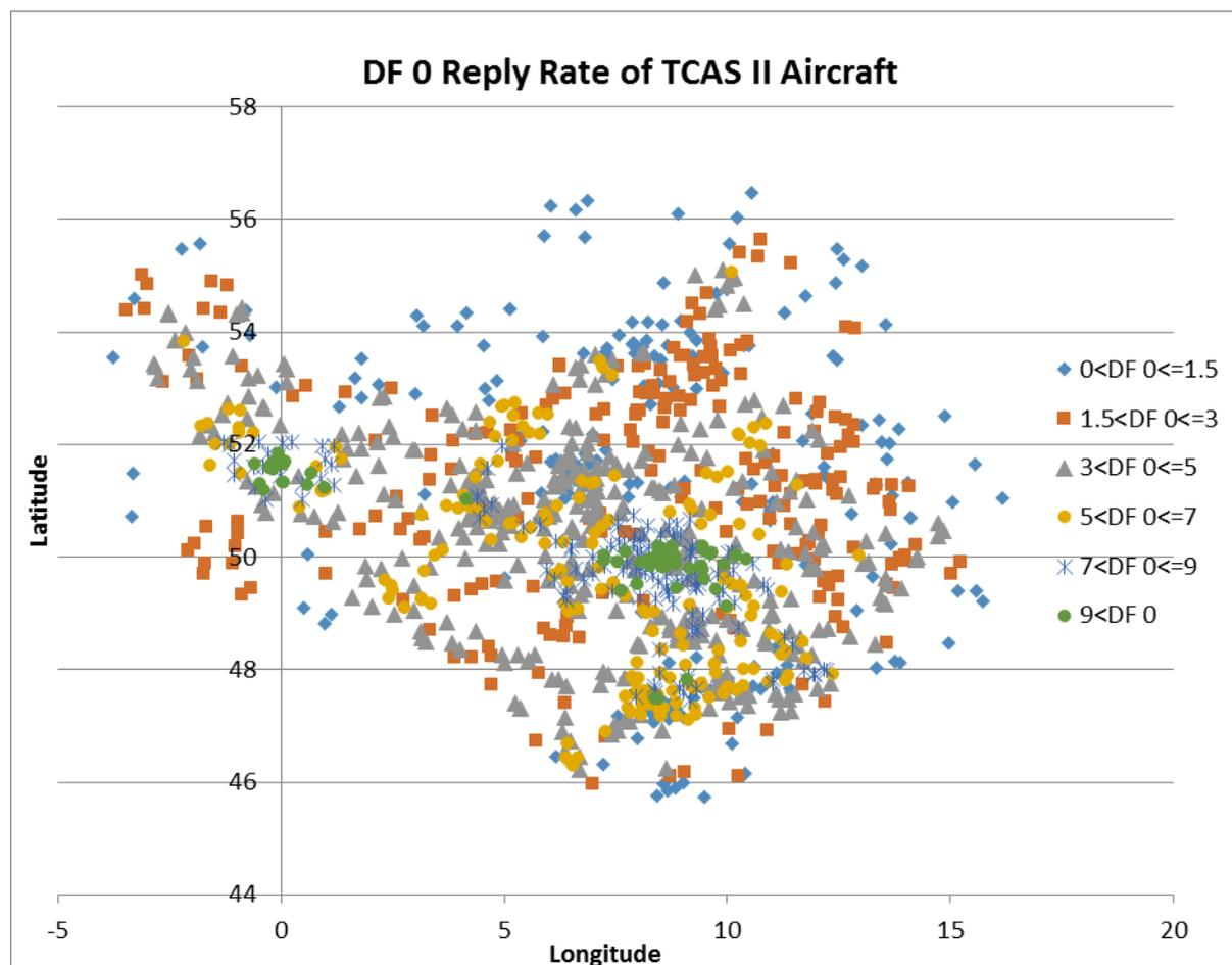
**Figure 25: DF 0 Reply Rate of TCAS II Aircraft (Horizontal View)**
