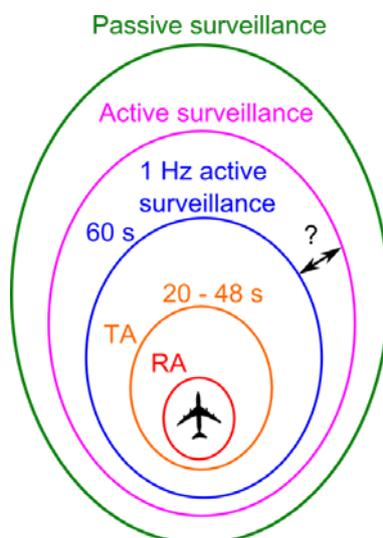
**Figure 11: Alert and surveillance zones around the own ship.**
