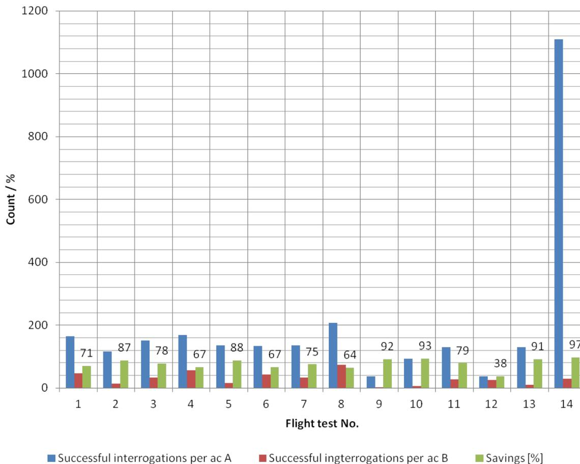
**Figure 32: Average number of successful replies per aircraft for samples A and B and the savings (labelled).**
