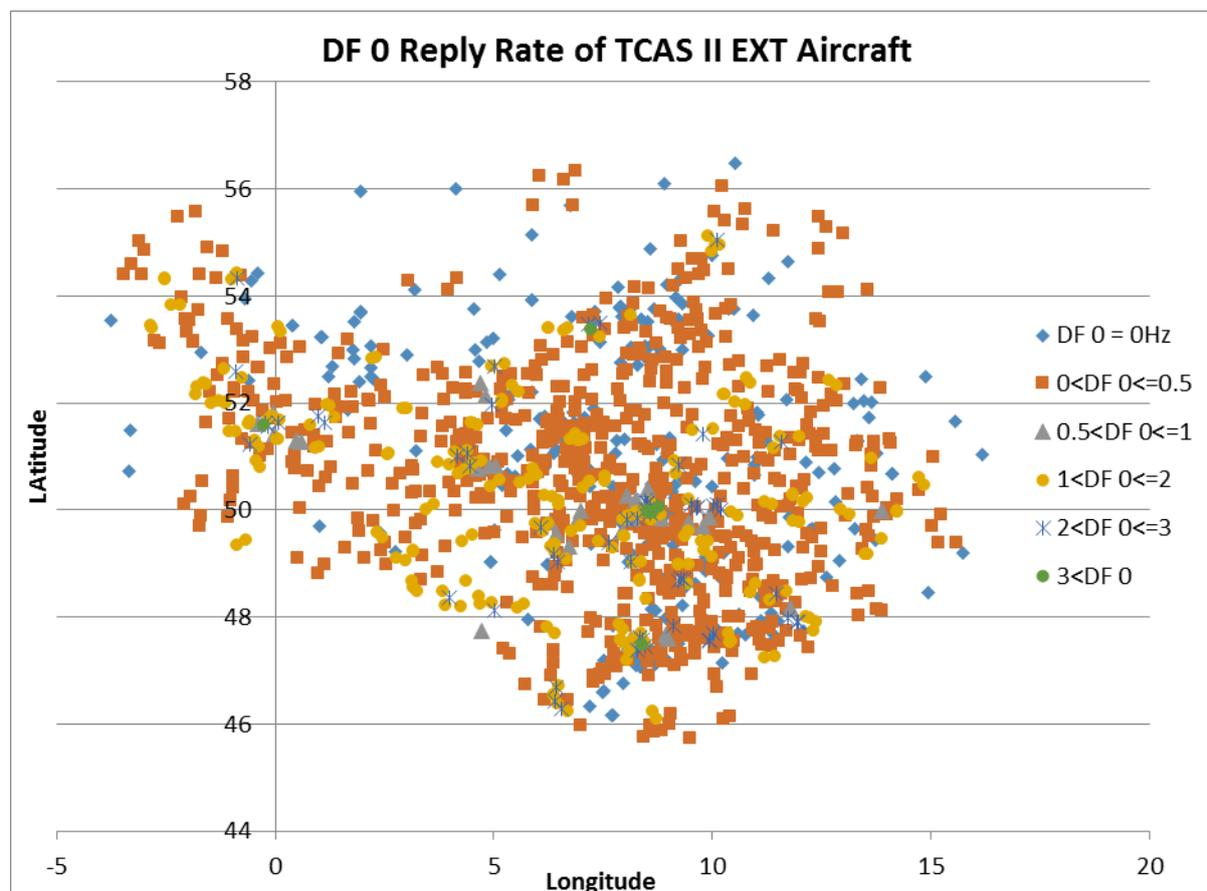
**Figure 26: DF 0 Reply Rate of TCAS II EXT Aircraft (Horizontal View)**
