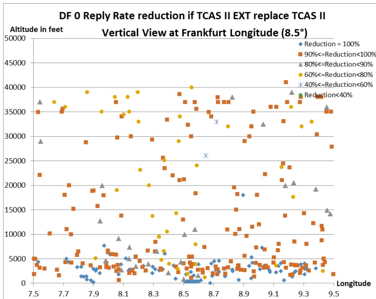
Figure 30: DF 0 Reply Rate Reduction around Frankfurt (Vertical View)
