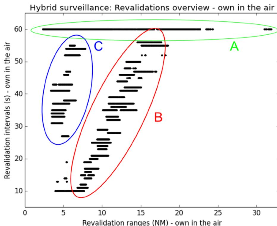
Figure 9: Relation between revalidation intervals and ranges (roof top testing, own in the air).
