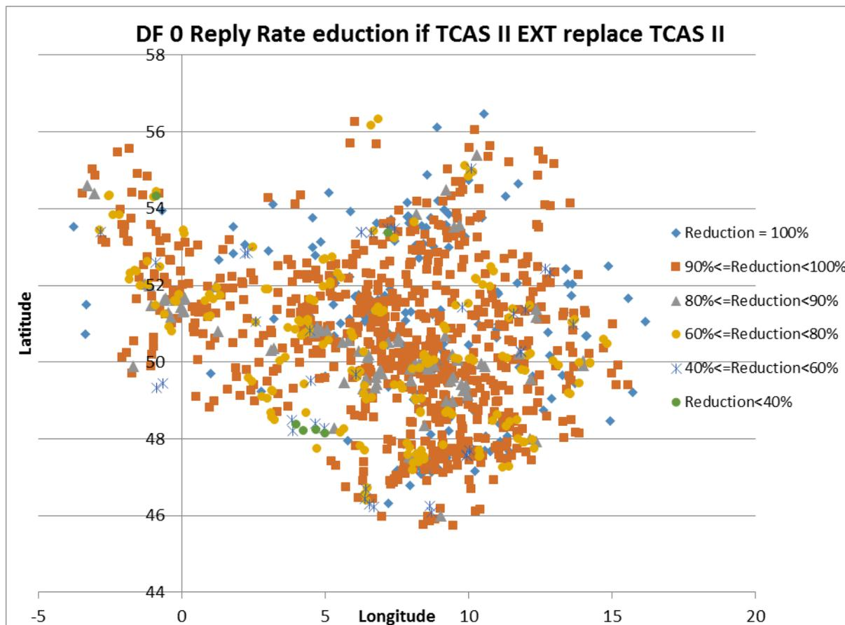
Figure 27: DF 0 Reply Rate Reduction (Horizontal View)
