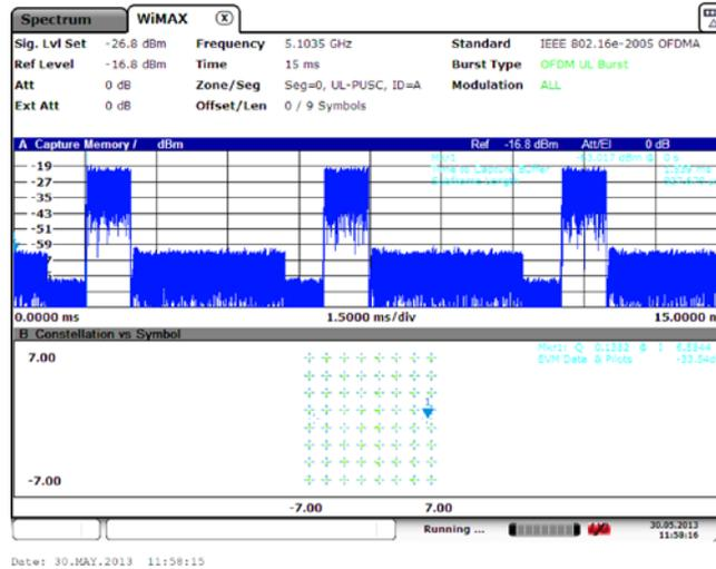
On the pictures above, measured frame duration is 5 ms (3 repetitions can be observed as the analysis time duration of spectrum analyzer is tuned to 15 ms). Detailed time measurements reveals an active DL Burst of 3,2 ms long and an UL burst of 1,5 ms long, consistent with ratio 32:15. The TDD nature of the frame is also clearly shown.
