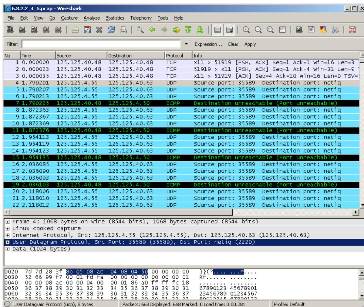
Figure 16: Wireshark Log on ASN-GW ports: no transmission for IP flow not compatible with the SF Classification for DL
