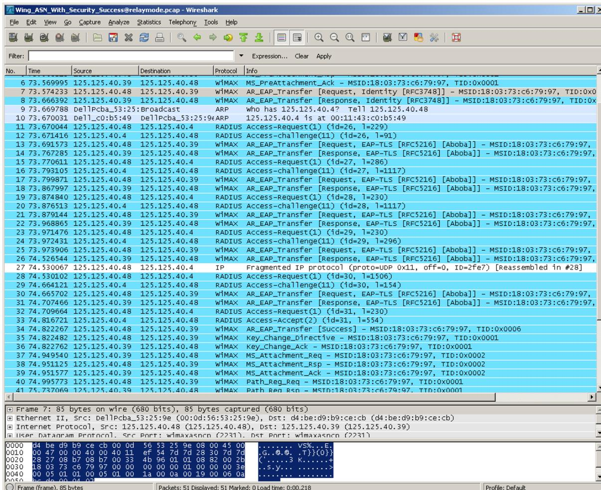
Figure 25: EAP-based Authentication Procedure
