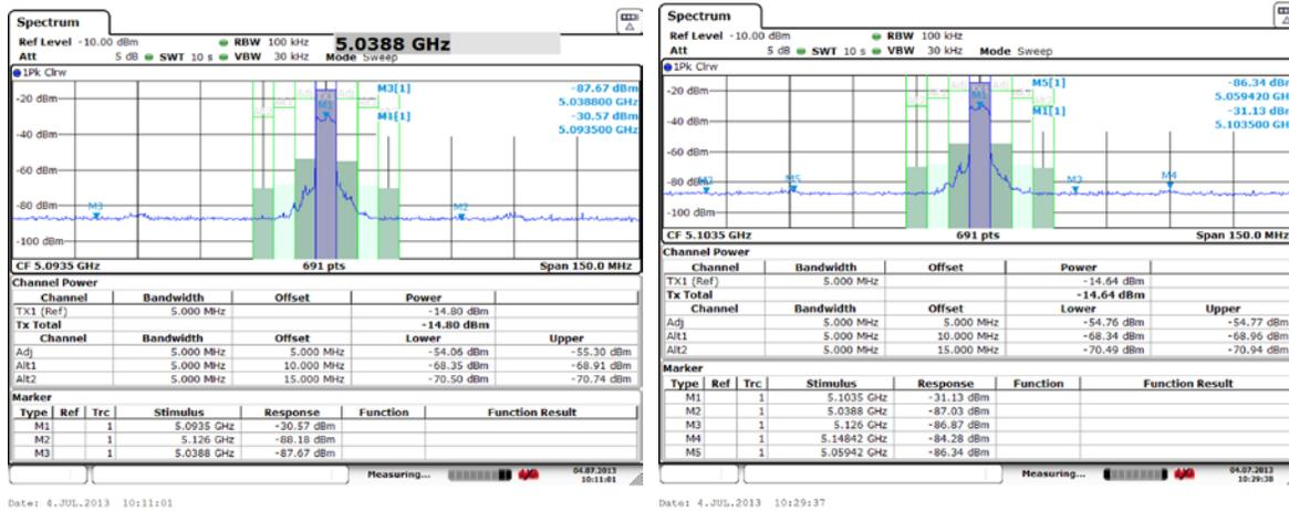
The maximum spurious level is at least 53 dB below the max. If we consider the BS emitting at 23 dBm over 5 MHz, this gives a level of 7 dBm in the RBW100 kHz corresponding to a level of spurious below -46 dBm in RBW 100 kHz.
