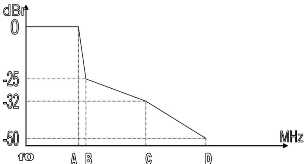
Figure 27: Selex AeroMACS BS prototype target spectrum mask
