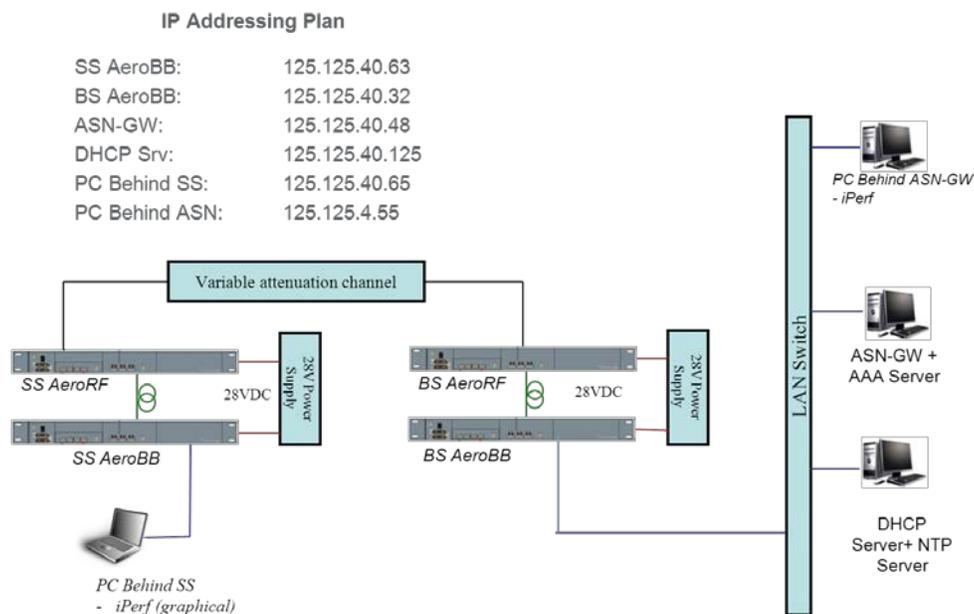
Figure 15: QoS - Test bed
