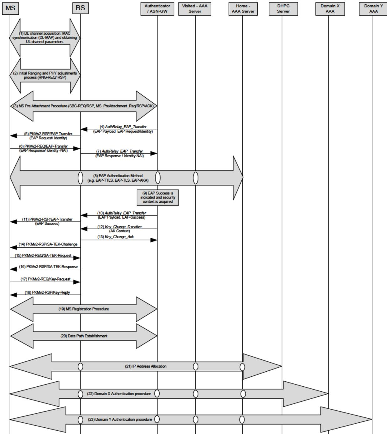
Figure 12: Initial Network Entry Time
