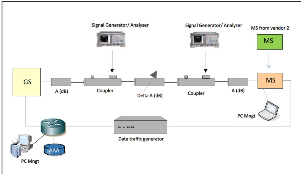
Figure 1: Lab\_test\_bed\_01 (Thales)
