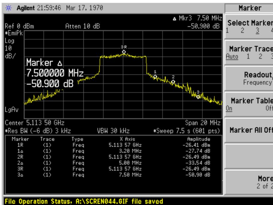
Figure 26: AeroMACS BS measured Spectral Mask
