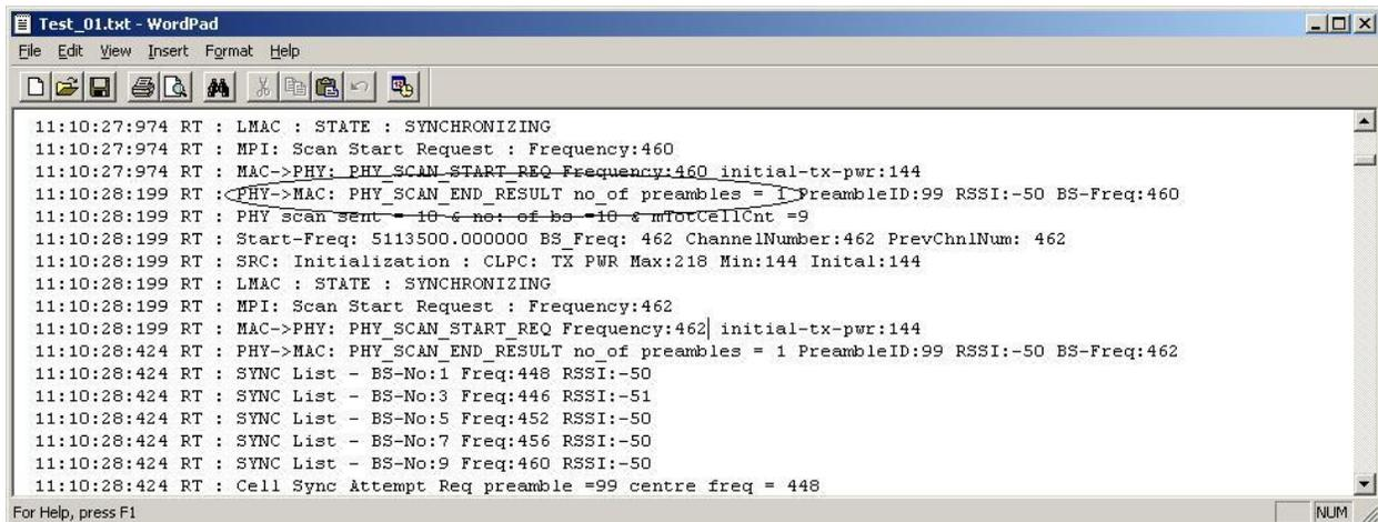
Figure 7: Preamble Detection by MS
