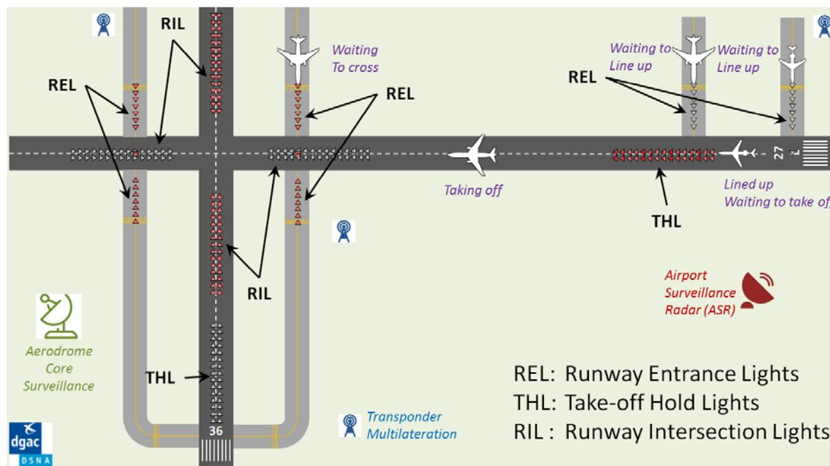
**Figure 4 – Different sets of lights part of the RWSL Solution Conflicting ATC Clearances detection (CATC)**
