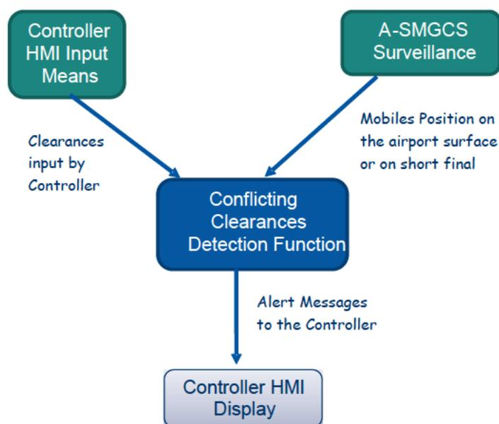
Figure 7 – Conflicting ATC clearances detection – Functional architecture
