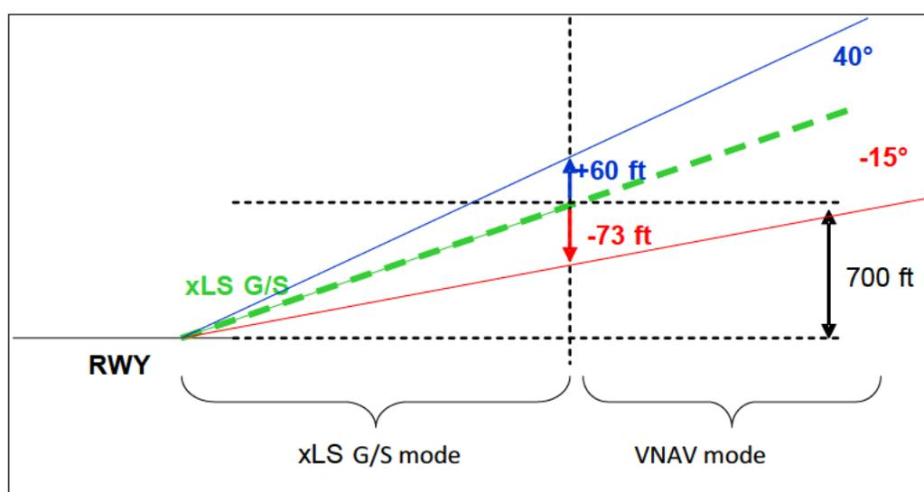
**Figure 5 : Vertical path with baro-referenced altitude in delta-ISA conditions**
