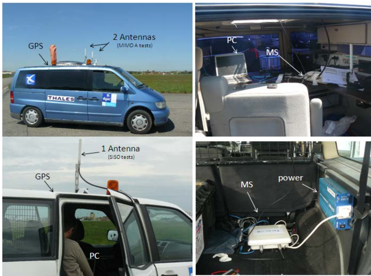
Figure 7-32: 2 DGAC Vehicle installation with 2 Thales MS
