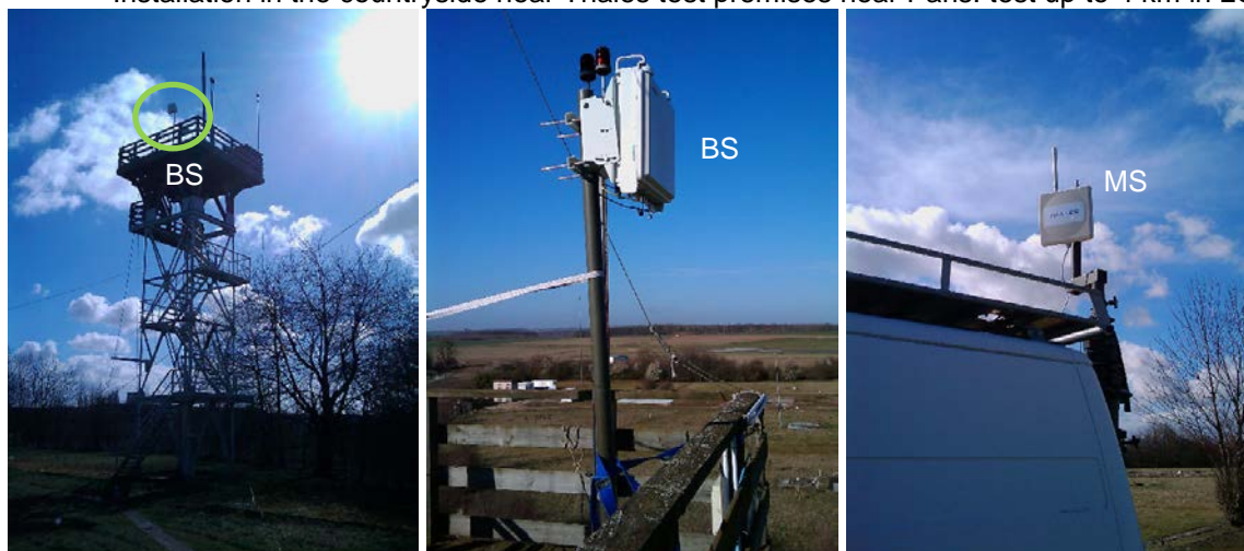
Figure 7-26: Setup of the BS on a tower and MS on a truck for outdoor tests
