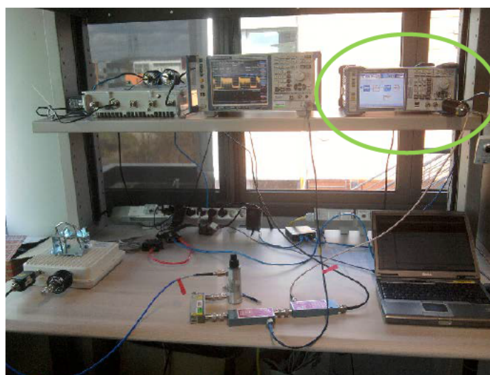
Figure 7-22: test bed configuration with a signal generator
