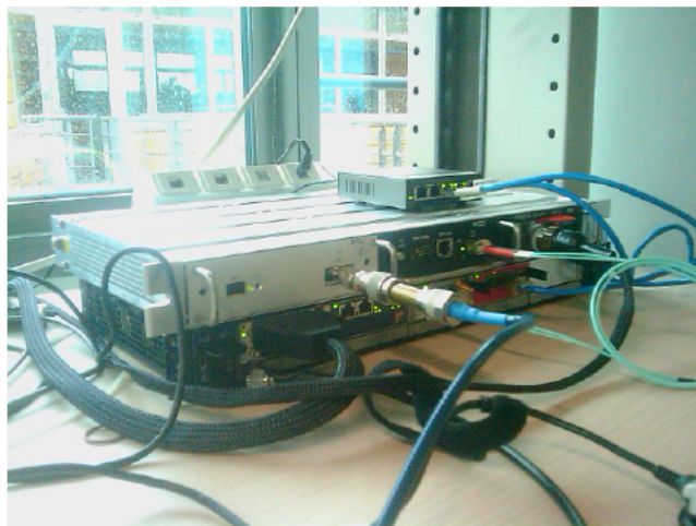
Figure 7-23: Selex MS in Thales lab (Baseband 1U rack below and RF 1U rack above)
