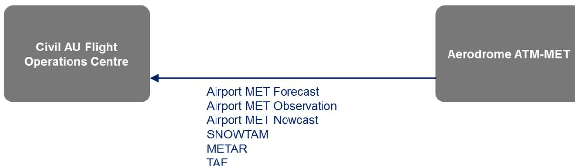
**Figure 7: Interoperability between the FOC and the Aerodrome ATM-MET Capability Configuration**
