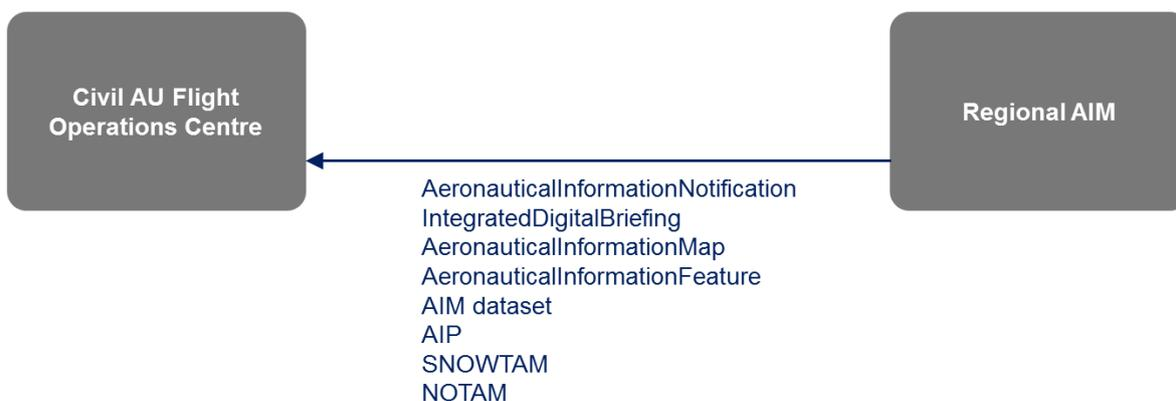
**Figure 11: Interoperability between the FOC and the Regional AIM Capability Configuration**
