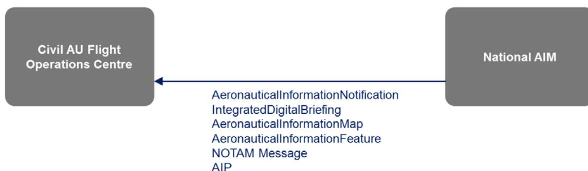
**Figure 10: Interoperability between the FOC and the National AIM Capability Configuration**
