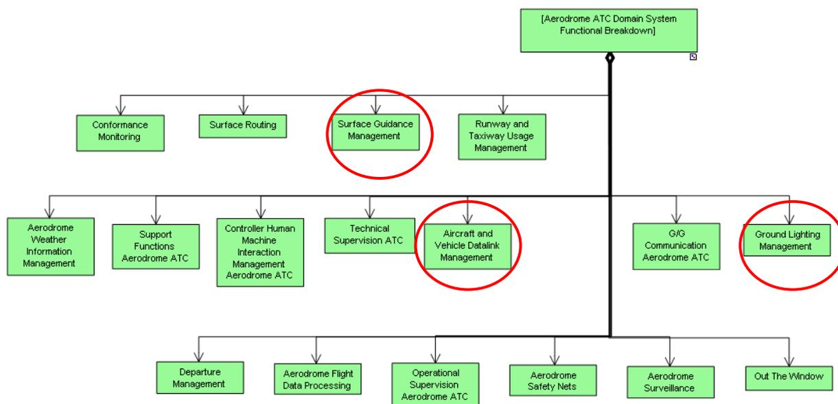
Figure 4: Aerodrome ATC Domain System - Functional Breakdown
