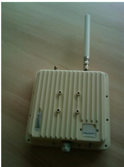
**Figure 12: Mobile Station equipped with a collinear antenna**
