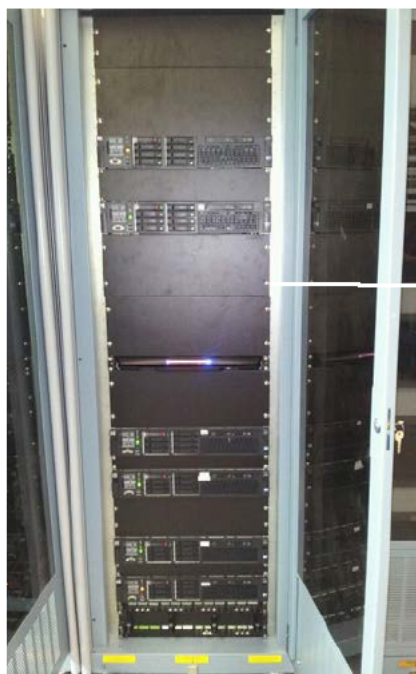
Figure 9: P15.04.05 SELEX ADS-B GS Prototype rack
