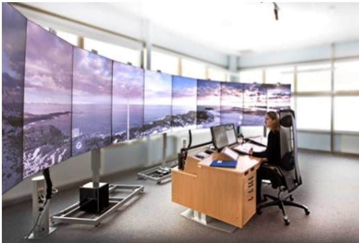
Figure 1 – Image from the platform validated in VP-058 for remote provision of AFIS to Værøy Heliport from Bodø remote tower centre
