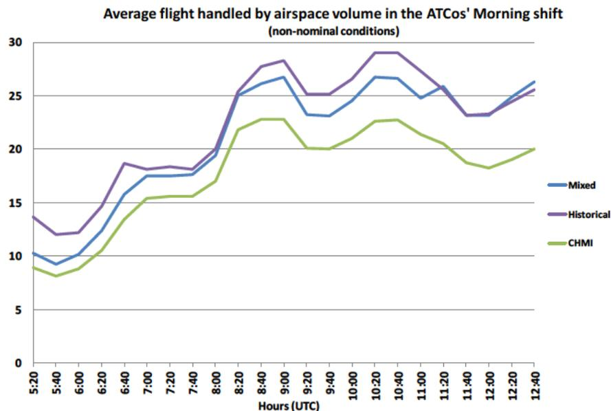
Figure 22: Number of flights able to enter airspace volume in the ATCos' Morning Shift (non-nominal conditions)
