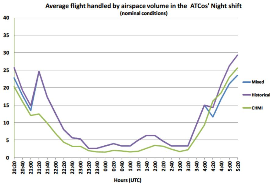
Figure 19: Number of flights able to enter airspace volume in the ATCos' Night Shift (nominal conditions)
