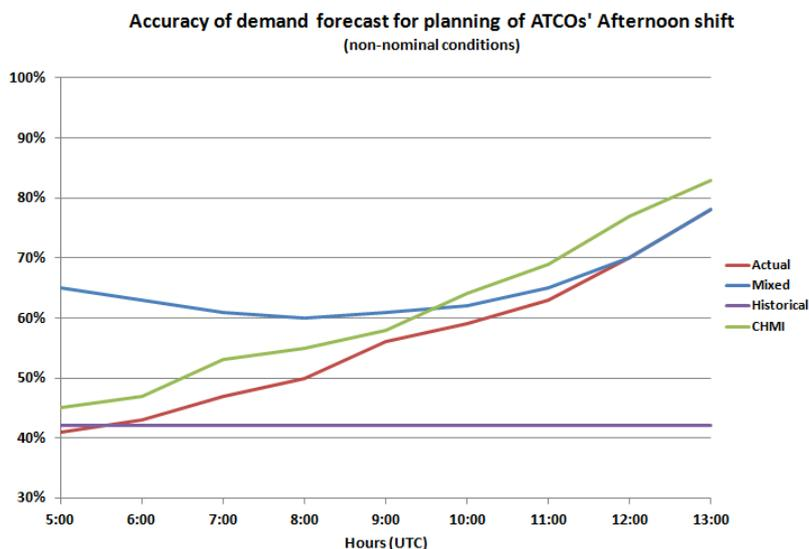
Figure 9: Demand forecast accuracy for the ATCOs' afternoon shift (non-nominal conditions)
