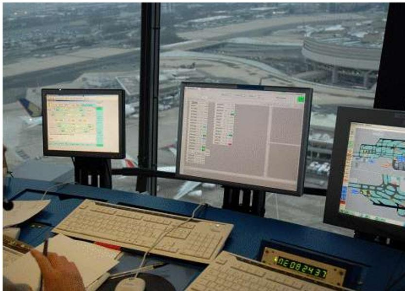
217 Figure 20: CDG - Clearance Delivery working position with the DMAN HMI in the centre
