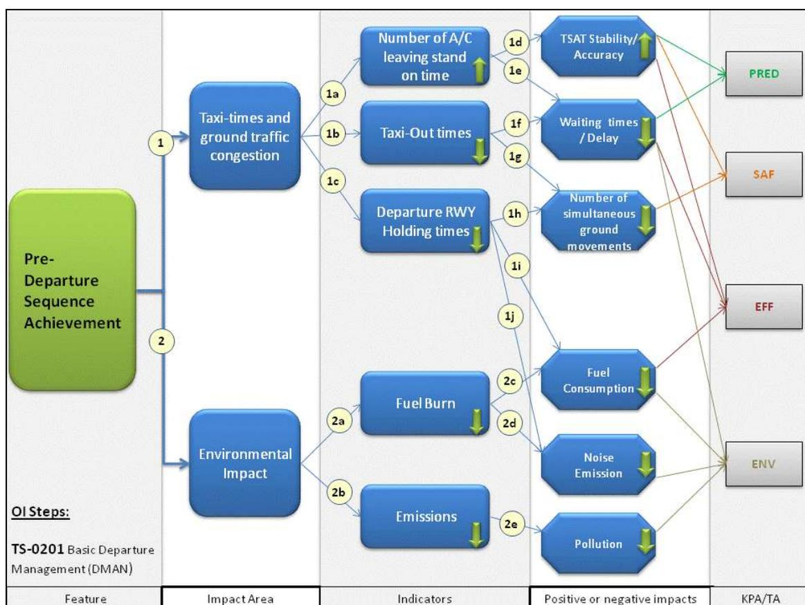
Figure 1: Basic DMAN Benefit Mechanisms Diagram
