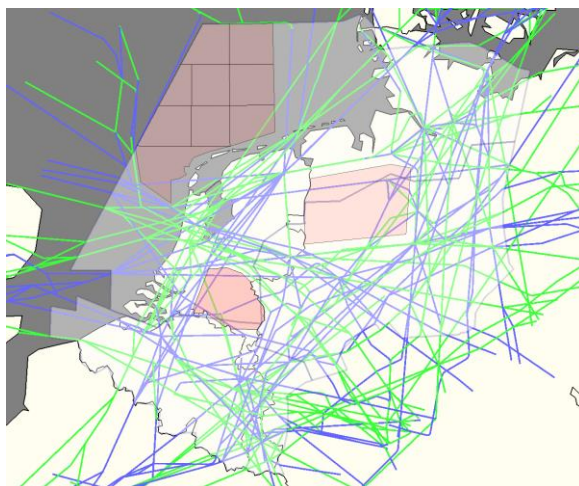
Figure 15: Active AMC avoided by DCTs using anchor points
