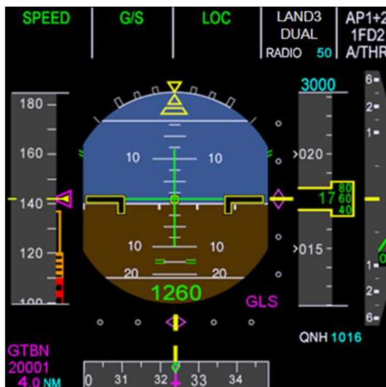
Figure 10: Monitoring GLS final approach on PFD
