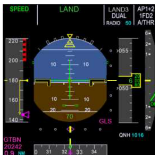
Figure 11: PFD without G/S deviation at 70ft RA
