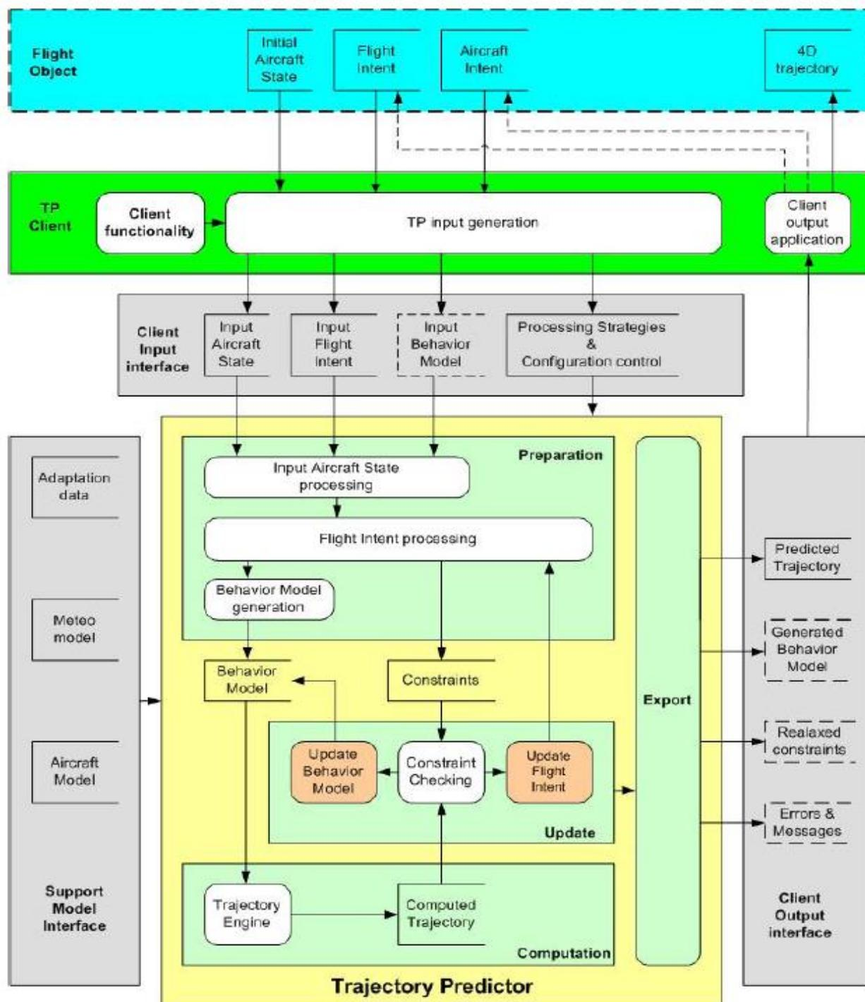
Figure 1: Trajectory Prediction – Data View (Source AP16)
