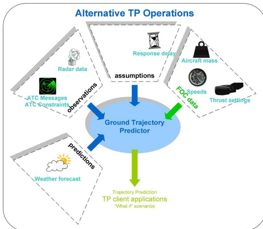
Figure 3: Alternative system (ground TP using AOC data)
