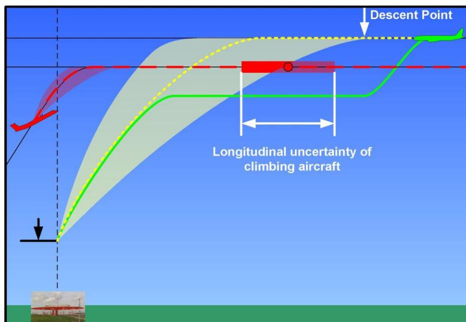
Figure 5: Descent planning using current TP
