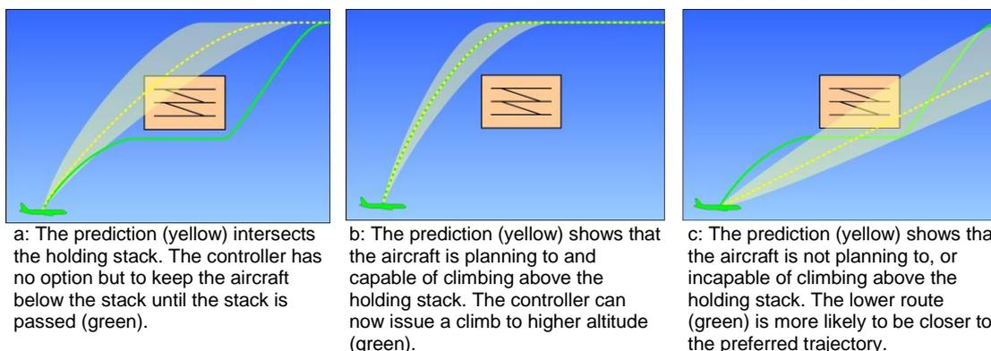
Figure 4: Effect of operator input in TP on controller selection of climb options
