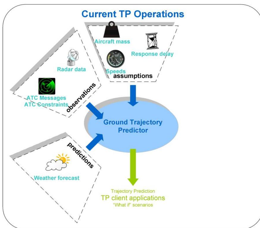
Figure 2: Current system (ground TP)
