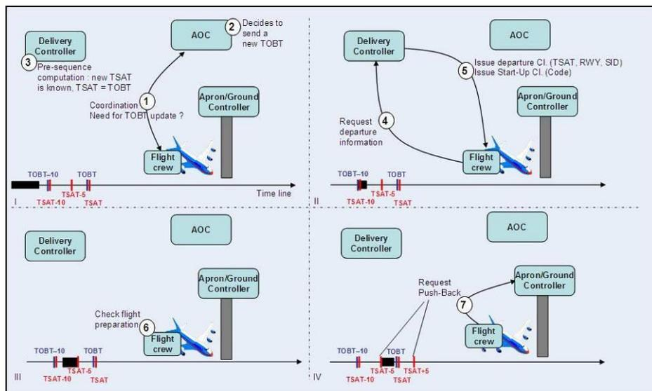
Figure 7: UC1 - Operational view – VHF Clearance
