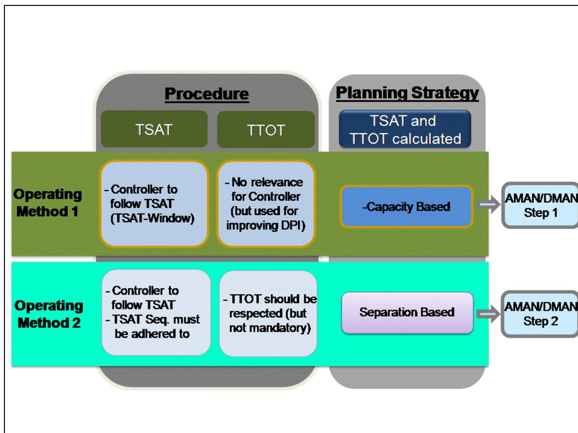
Figure 6: Operating Methods illustration
