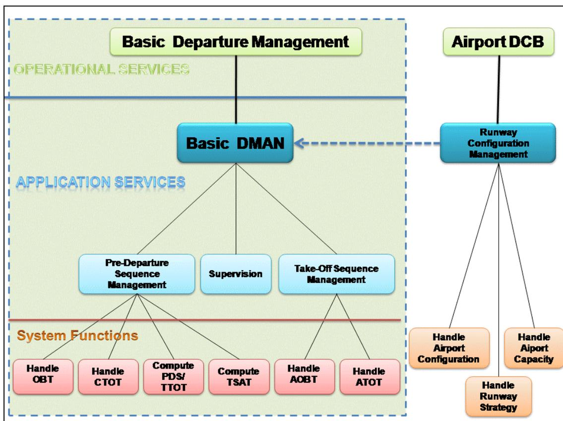
Figure 3: Basic DMAN Services and system functions
