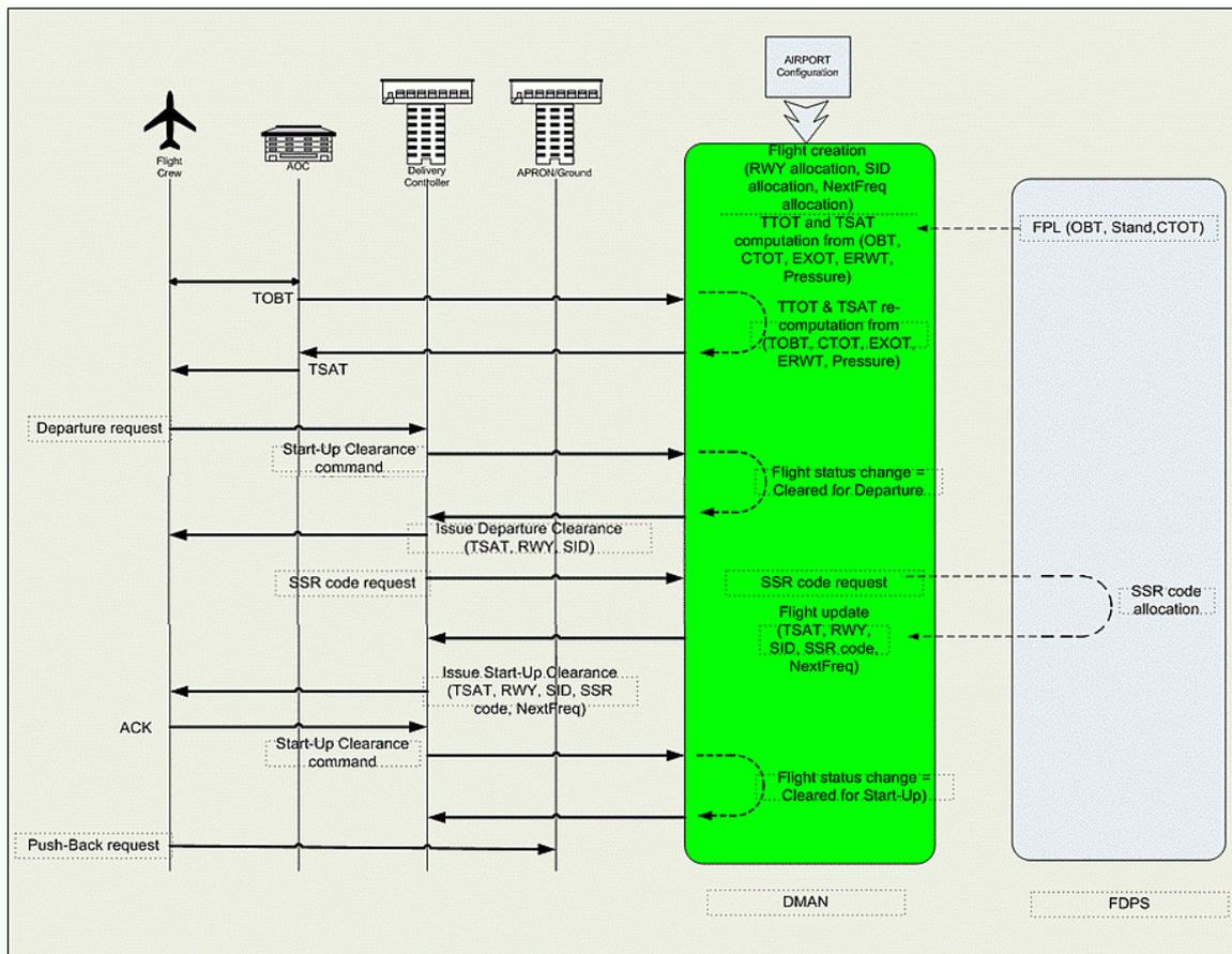
Figure 8: UC1 - Transactional view – VHF Clearance
