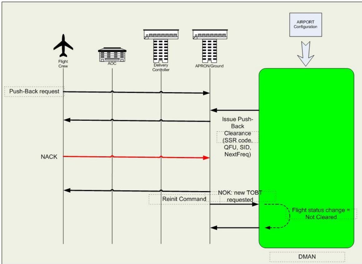
Figure 26: UC12 – Transactional view (Case 1: Flight is not ready)
