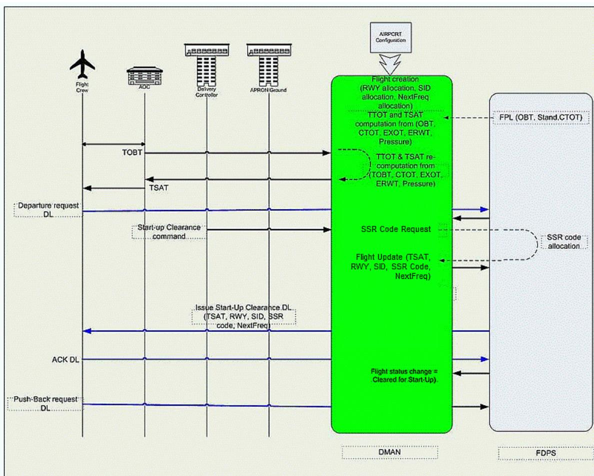
Figure 9: UC1 - Transactional view – Datalink Clearance
