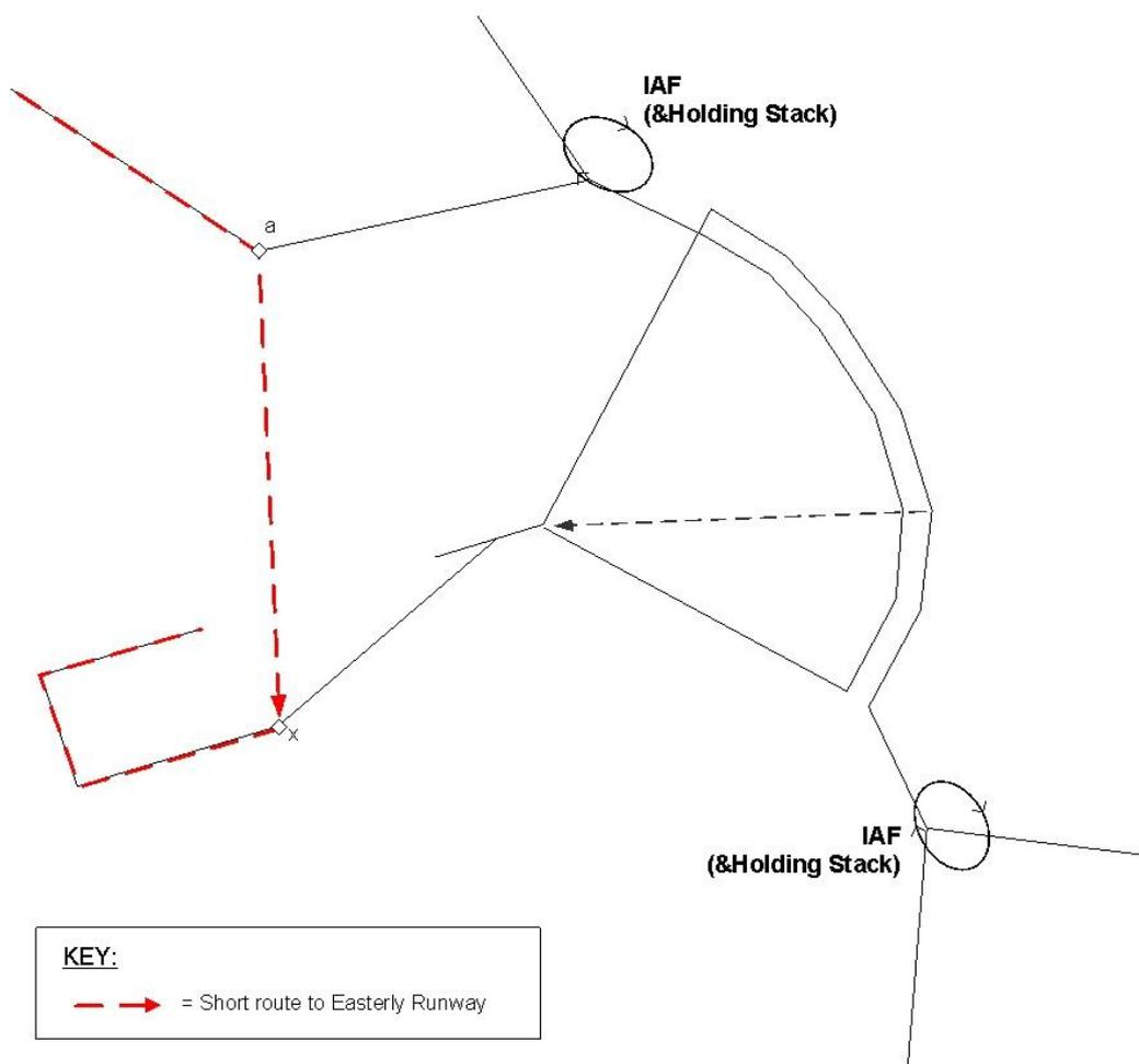
Figure 6: Example of a short route for an Invariant Point Merge Design
