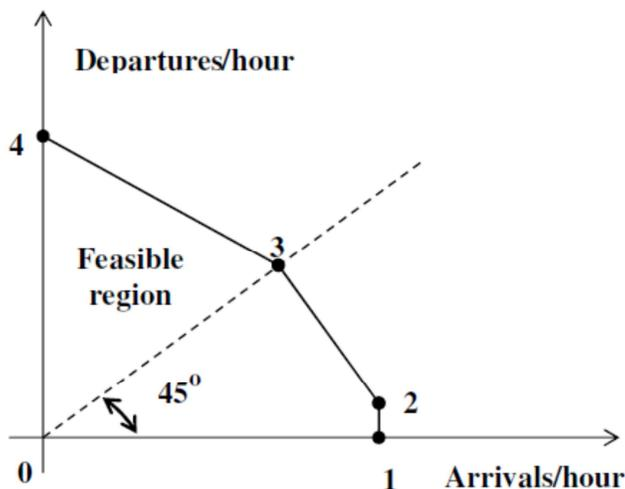
Figure 8: Capacity envelop for a single runway (source [20])
