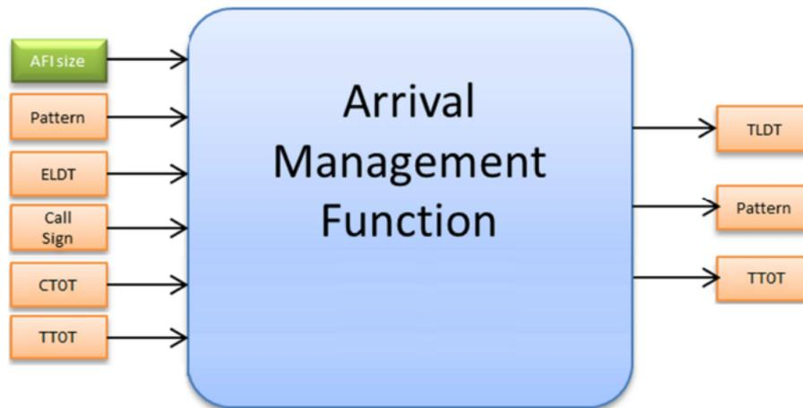
Figure 3: Arrival Management Function - input/output model
