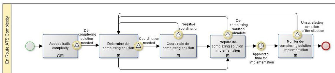
Figure 2: Traffic Complexity Process Diagram
