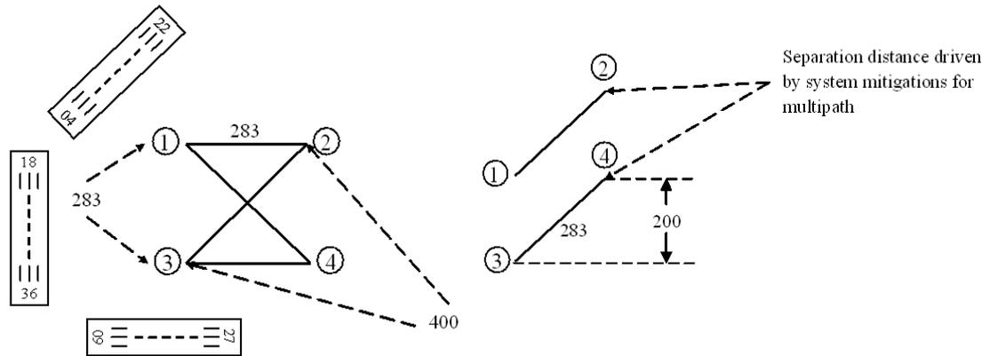
**Figure 5-24: GBAS Reference antenna layouts for spatial ionospheric monitoring [26]**
