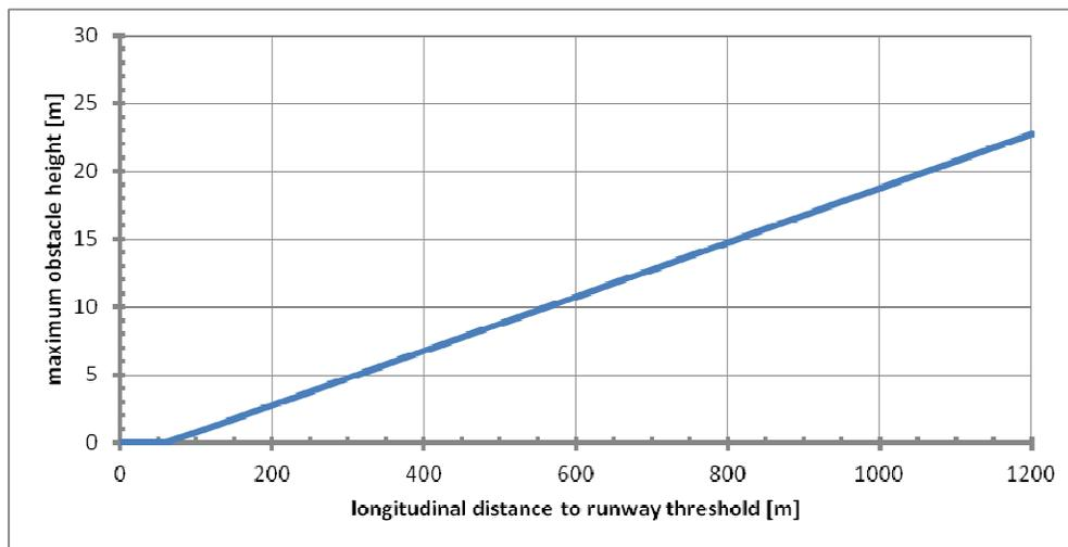
**Figure 4-4: Maximum obstacle height underneath the approach path as a function of distance from runway threshold for a CAT II/III runway**
