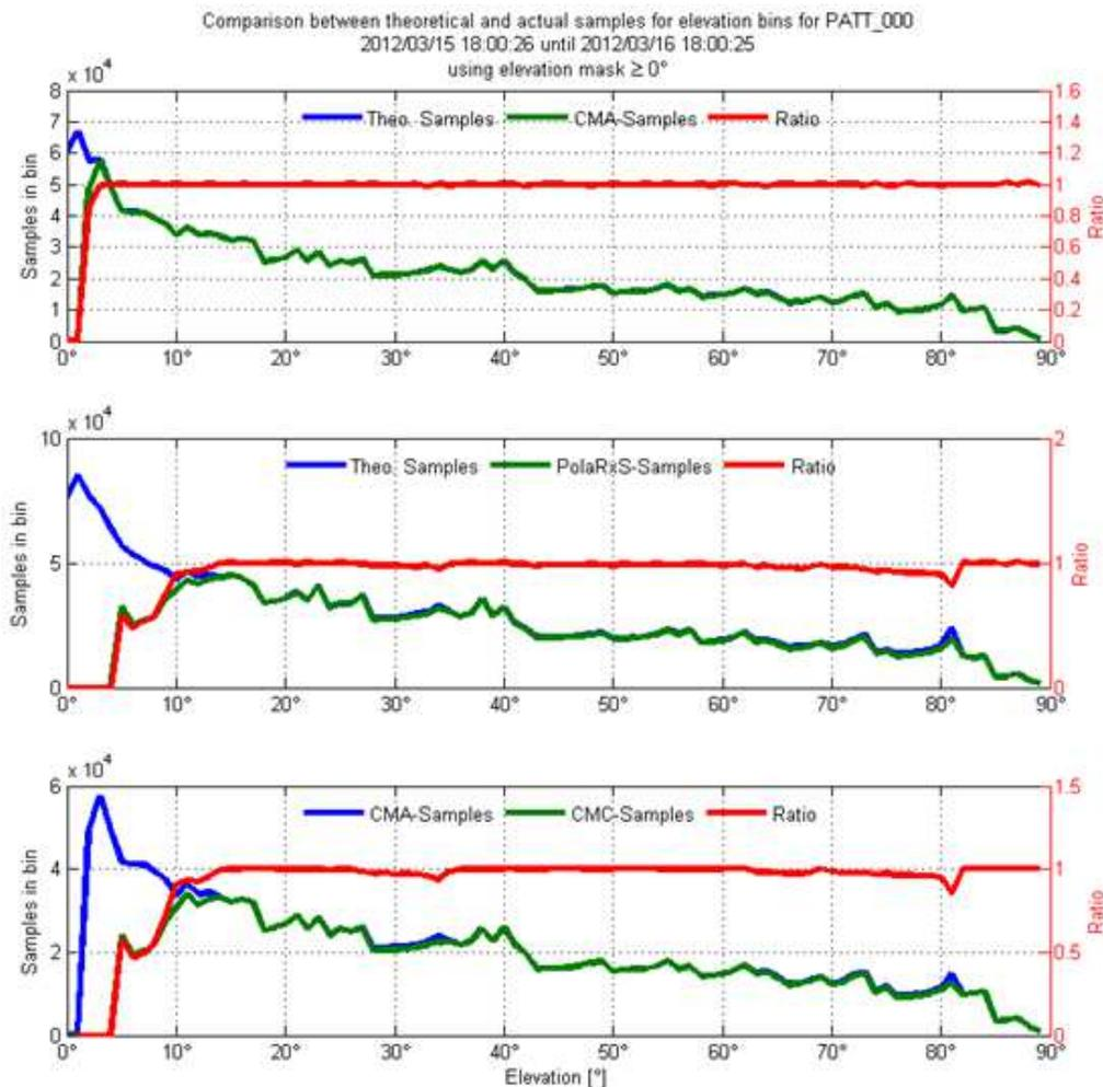
**Figure 5-7: Example of Number of samples used for RMS(CMC) evaluation. The different figures represent the different measurement data sources (compare to [56])**
