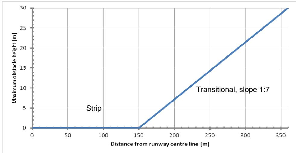
**Figure 4-3: Maximum obstacle height as a function of distance from runway centre line for a CAT II/III runway**
