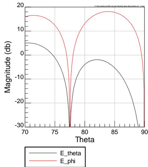
**Figure 5-15: Radiation Pattern with phase centre  $2 \lambda$  (5-6m) over ground plane**
