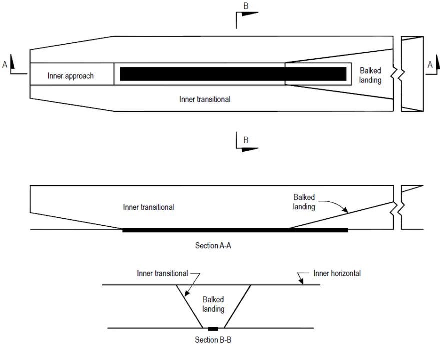
Figure 9-2: Inner approach, inner transitional and balked landing obstacle limitation surfaces
