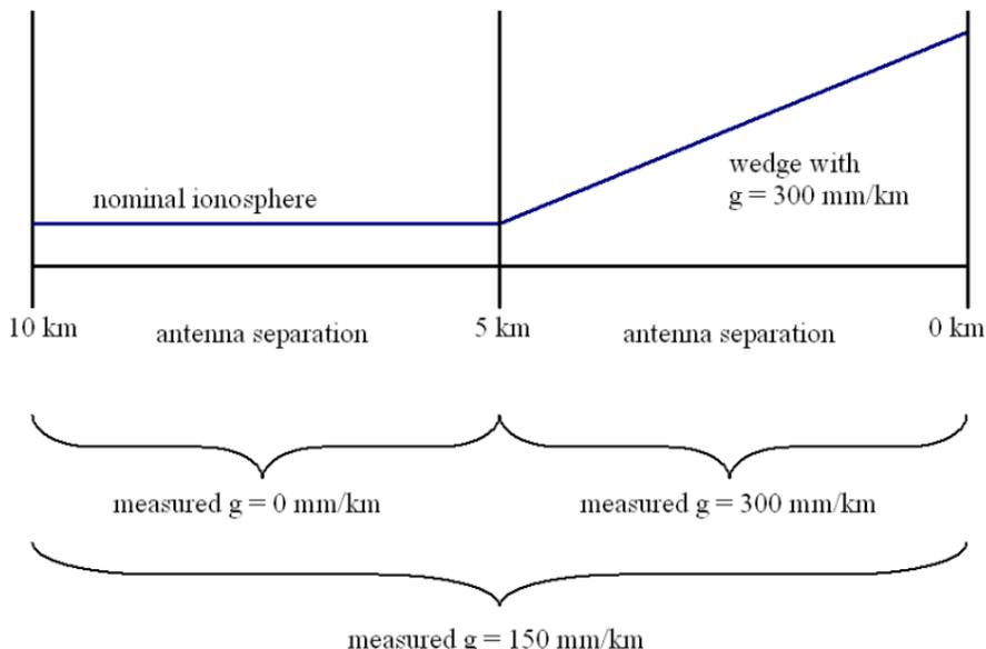
**Figure 5-21: Potential problem for antennas which are separated more than five kilometers**
