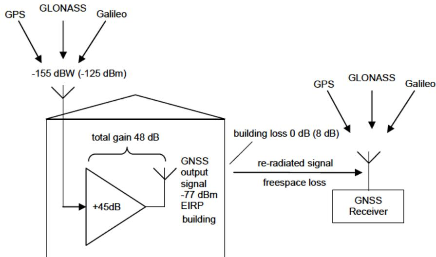
Figure 5-3: Proposed European technical standard for GNSS repeaters
