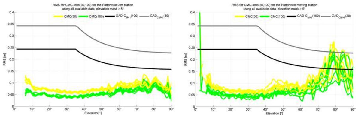
**Figure 5-6: Example of RMS(CMC) vs. Elevation angle plot. Each curve represents the measurement result for one day (compare to [56])**
