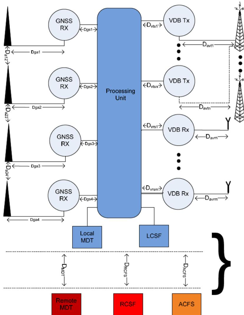
Figure 4-1: Manufacturer specific separation distances
