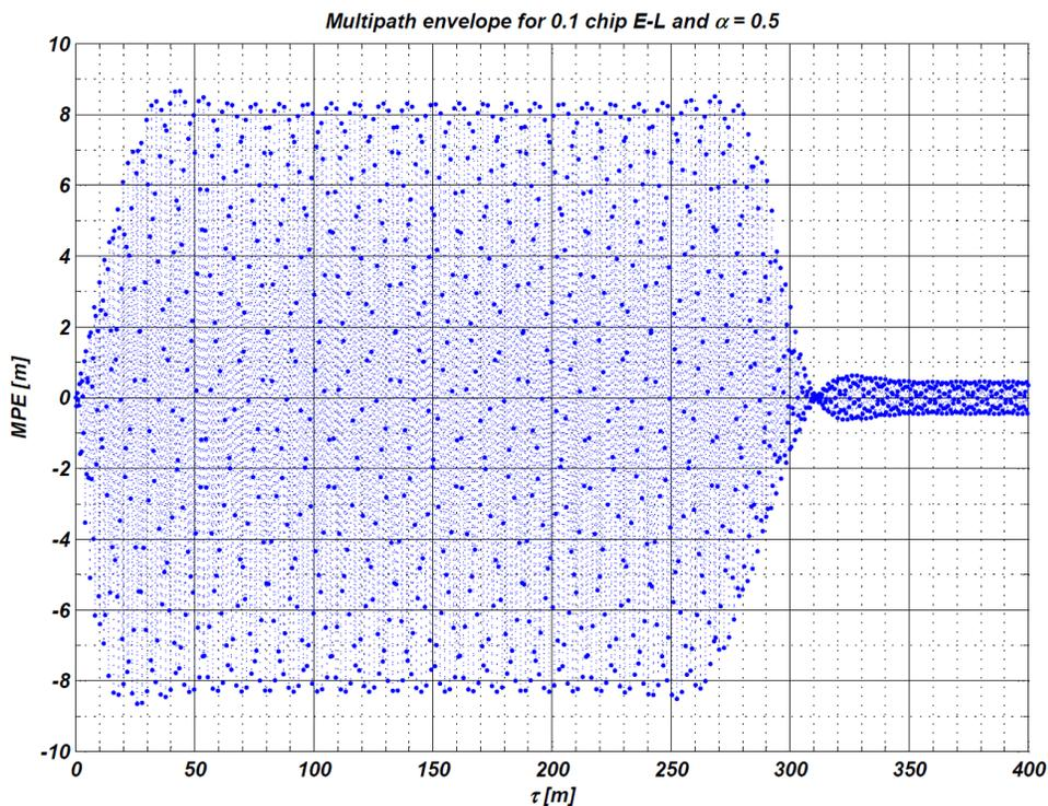
**Figure 5-4: Example of the range of resulting multipath errors for a narrow correlator receiver incl. pre-correlation filter influence and assuming a reflection coefficient of 0.5, simulated for PRN22.**
