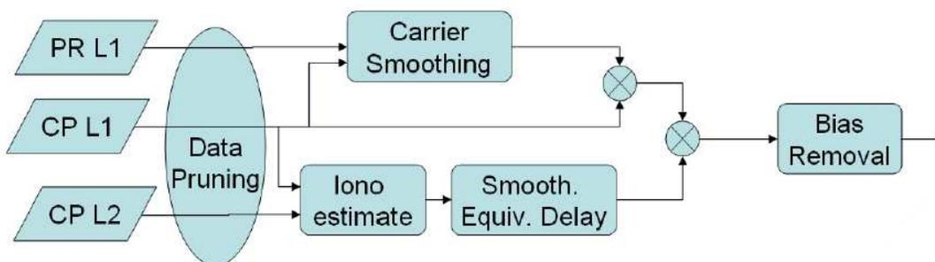
Figure 5-5: Determination of the CMC Observable [48].
