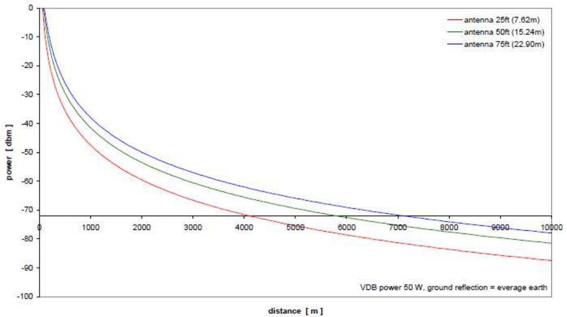
**Figure 5-13: VDB Simulation results at 8ft (2.4m)**
