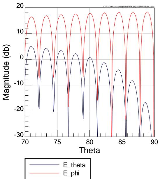
**Figure 5-16: Radiation Pattern with phase centre  $12 \lambda$  (28-34m) over ground plane**
