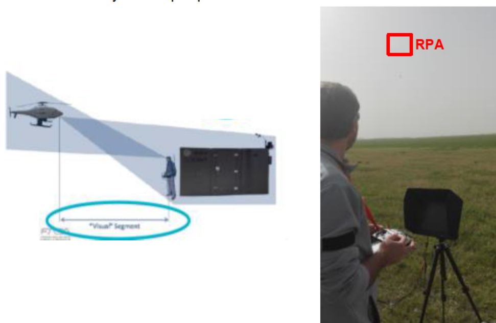
Figure 4.1-2 Validation of video communication among external pilot and RPA
