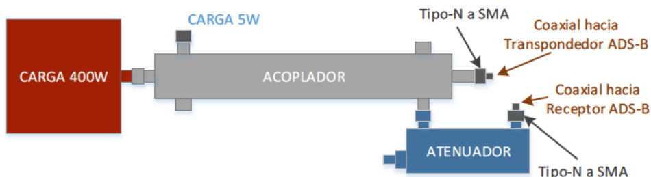
Figure 4.1-19 Scheme of the RF connections for the ADS-B transponder test set-up
