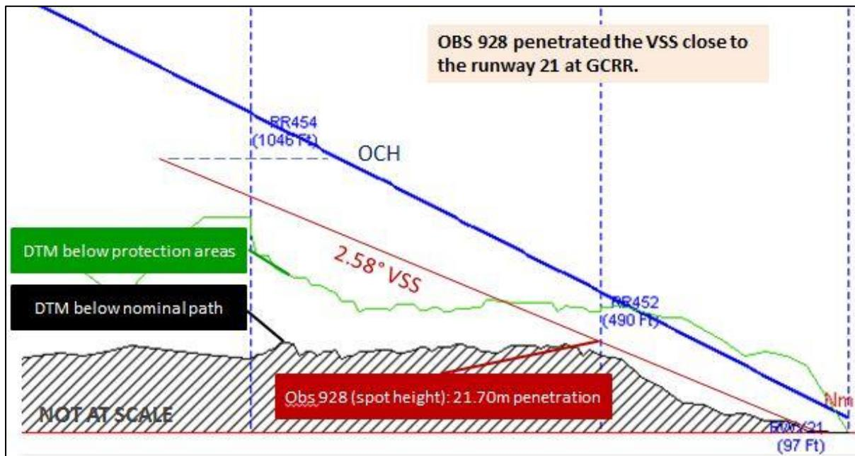
Figure 20 - Detailed Design GCRR RNAV RWY 21 – VSS vertical view
