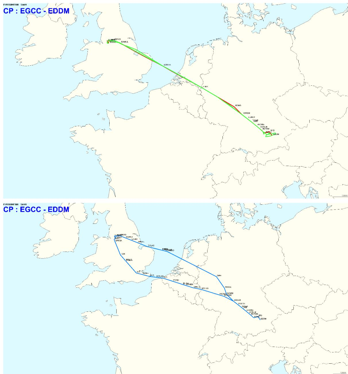
**Figure 65: User Preferred Routings EGCC – EDDM (top) and respective RAD-conform routings (below)**
