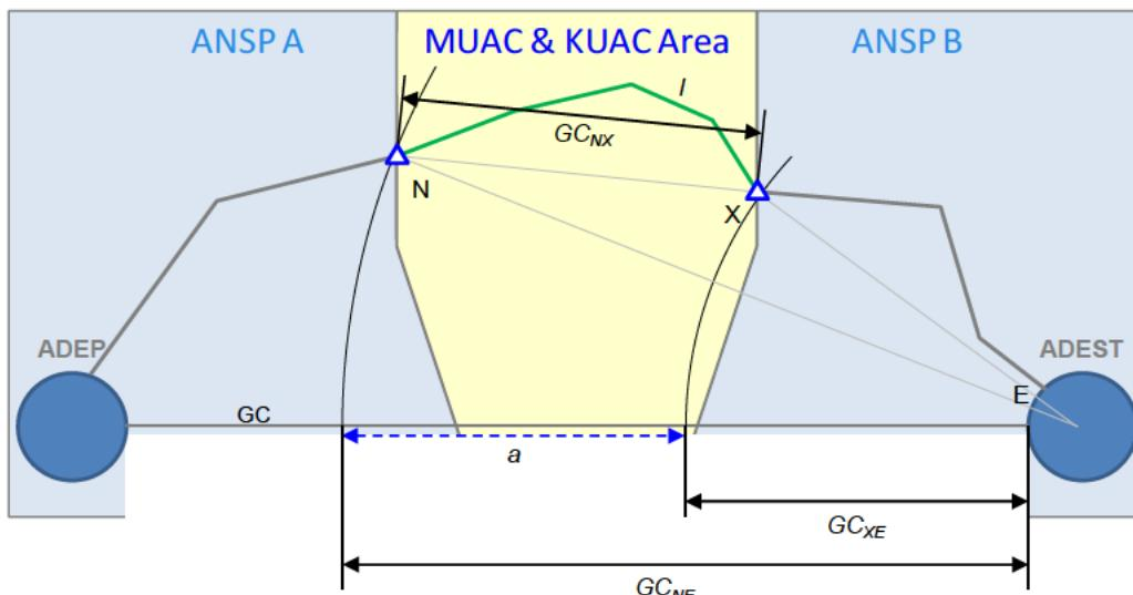
Figure 23: Geometric construction of Route Efficiency Indicators REDES and RESTR
