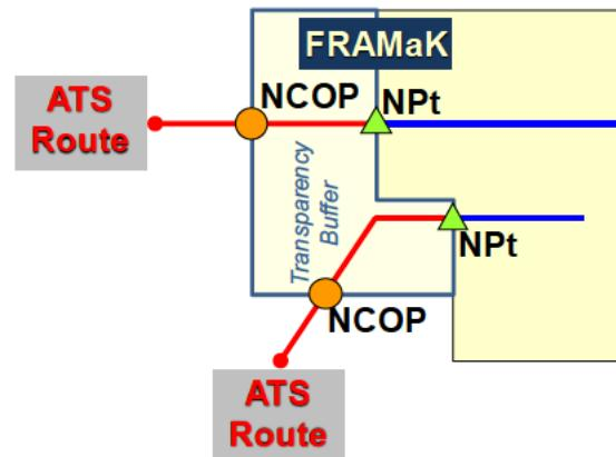
**Figure 7:** Transparency Buffer (vertical cut)
