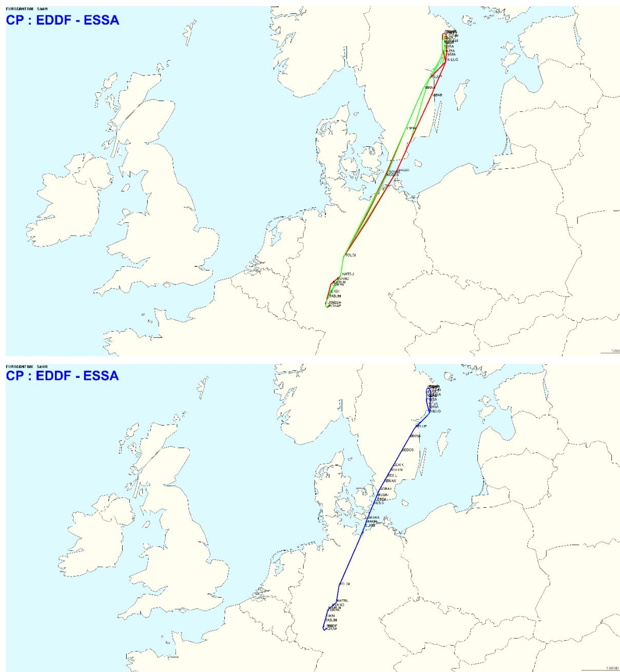
Figure 60: User Preferred Routings EDDF – ESSA (top) and respective RAD-conform routings (below)
