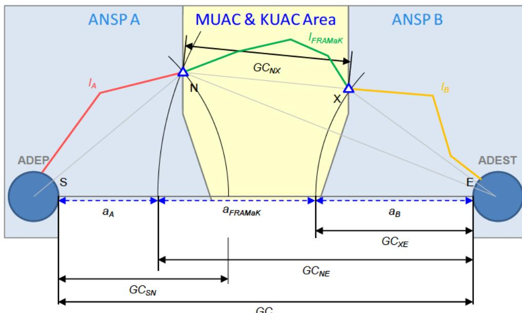
**Figure 24: Geometric construction of Route Efficiency Indicators REDES and RESTR considering the complete routing**
