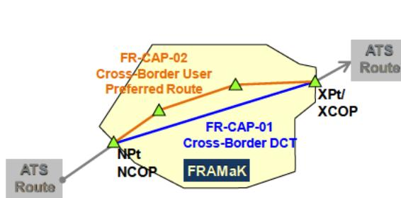
**Figure 4:** Schematic structure of FRAMaK Cross-Border DCTs and Cross-Border User-Preferred Routes (horizontal cut)
