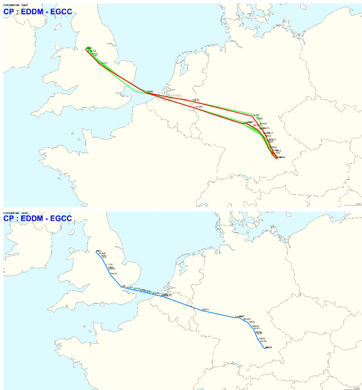
Figure 64: User Preferred Routings EDDM – EGCC (top) and respective RAD-conform routings (below)
