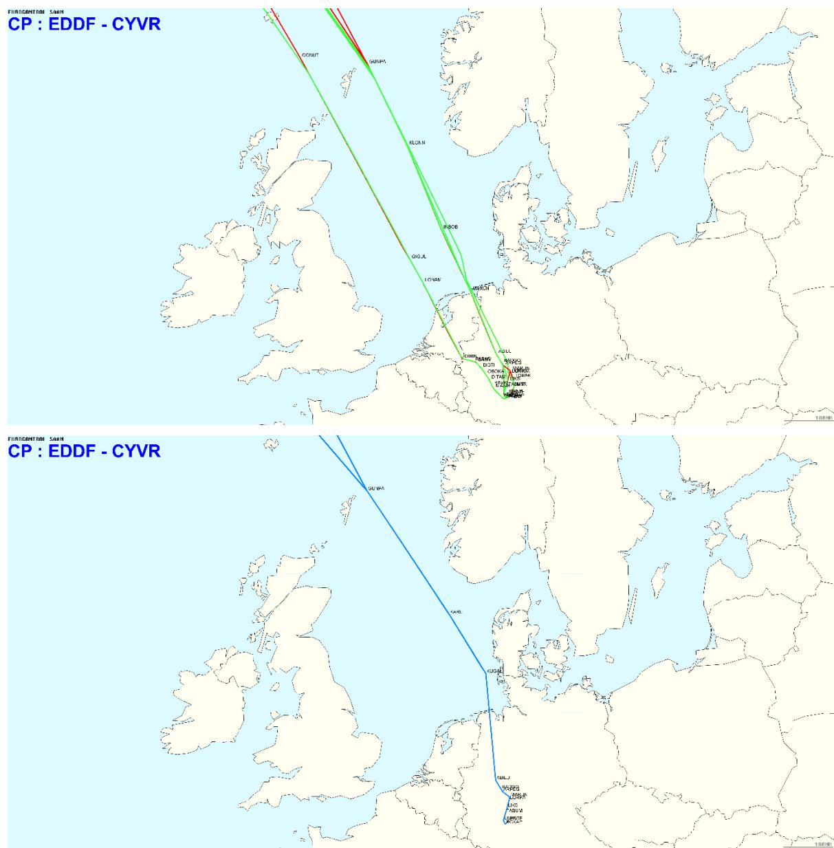
Figure 62: User Preferred Routings EDDF - CYVR (top) and respective RAD-conform routings (below)
