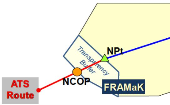
**Figure 6:** Transparency Buffer (horizontal cut)
