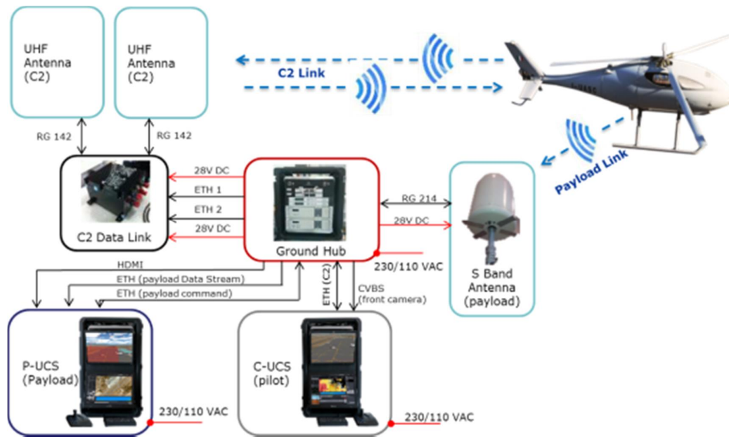
Figure 7: Flight system architecture overview
