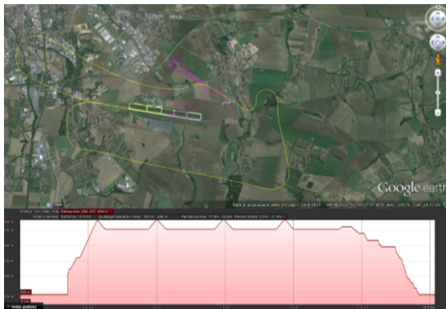
Figure 26: Flown RPA Mission (purple) and light aircraft trajectory (yellow) for Run#2.2 (in bottom the elevation profile of RPA mission)
