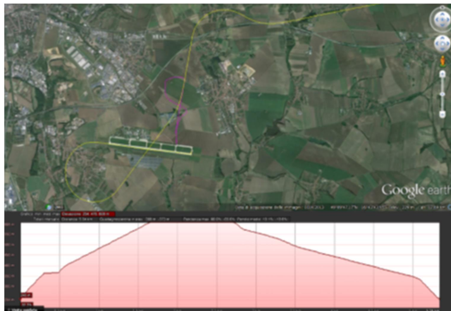
Figure 46: Flown RPA Mission (purple) and light aircraft trajectory (yellow) for Run#3.2 (in bottom the elevation profile of RPA mission) in Google Earth
