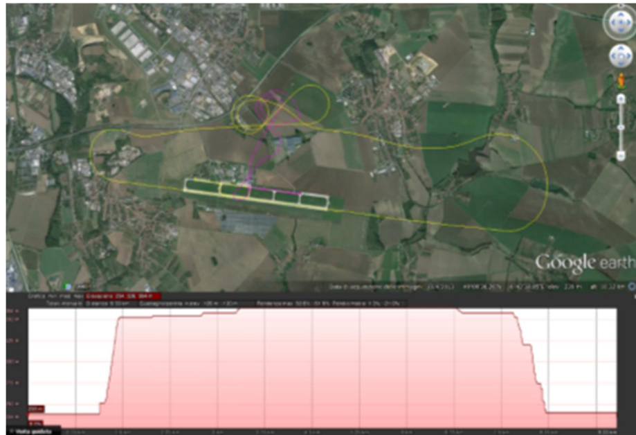
Figure 22: Flown RPA Mission (purple) and light aircraft trajectory (yellow) for Run#2.1 (in bottom the elevation profile of RPA mission)
