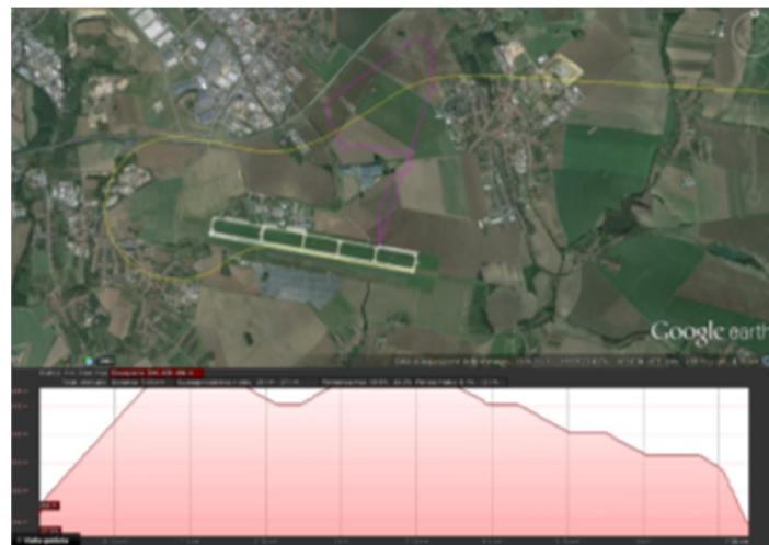
Figure 42: Flown RPA Mission (purple) and light aircraft trajectory (yellow) for Run#3.1 with observer (in bottom the elevation profile of RPA mission)
