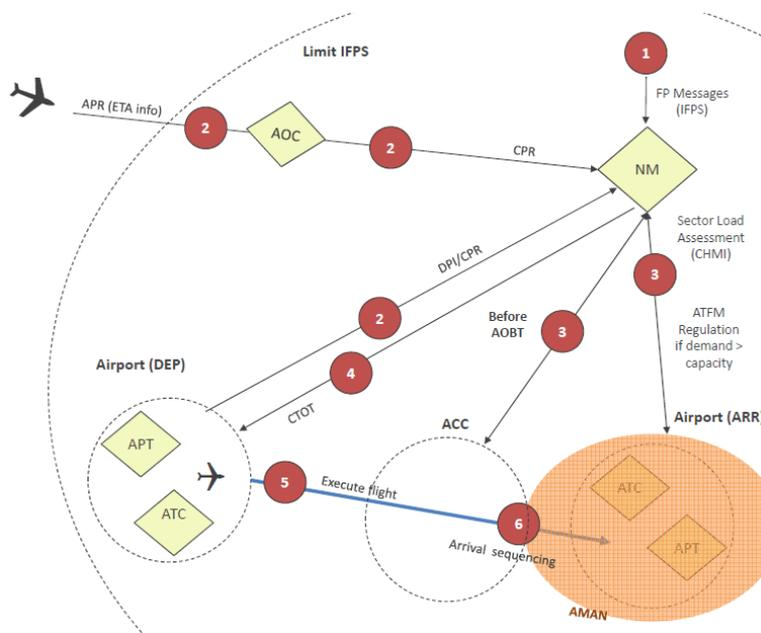
**Fig. 1: Information flow when destination airport/ACC are constrained**
