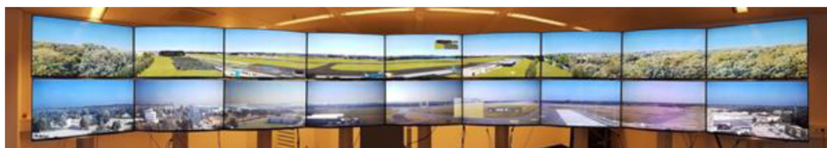
Figure 35: Multiple Remote Tower operation set-up with NARSIM simulation on top
