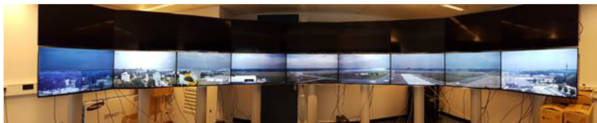
Figure 31: Single Remote Tower operation set-up for Groningen Airport Eelde
