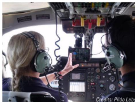
The SNI flight procedure under test was a Point In Space (PinS) LPV enabled by EGNOS and designed by Pildo Labs. It was flown by the Barcelona-based operator CatHelicopters using Pildo Labs' GNSS Flight Validation Platform, while the approach air traffic controllers from ENAIRE (former AENA) supported the trials too. The flight demonstrations were run as part of NASCIO, a SESAR demonstration project.
