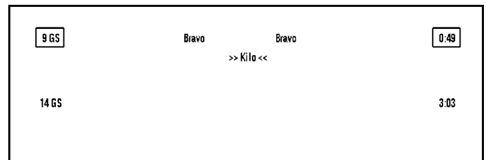
Figure 2. Speed and time information presented superimposed over the sky in the out-the-window airport view. (See text for description).
