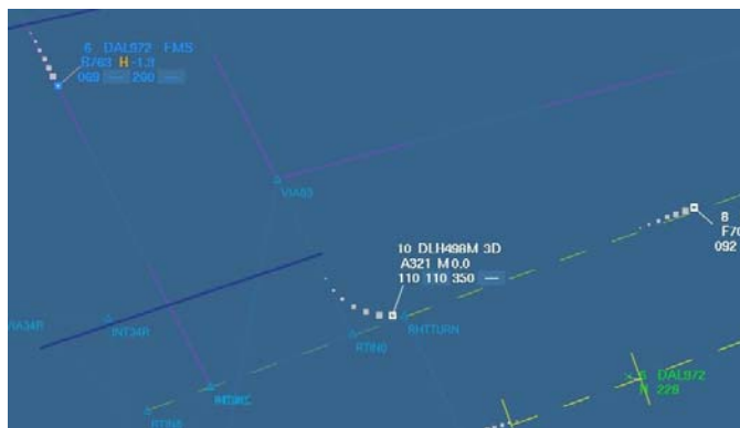
Figure 7. Screenshot of the HMI radar display with the blue reporting line on the left between the light blue displayed flight “DAL972” and the white flight “DLH498M”. The green label of flight “DAL972” on the bottom right is the projected ghost label on the final of the same flight on the upper left corner of the screenshot (sectional enlargement of Figure 5. ).
