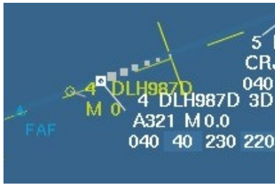
Figure 8. Screenshot of the HMI radar display with the labels of flight “DLH987D” (white) and its “target” (yellow). The target represents its ideal position on the final from the AMAN’s scheduling view (sectional enlargement of Figure 5. ).
