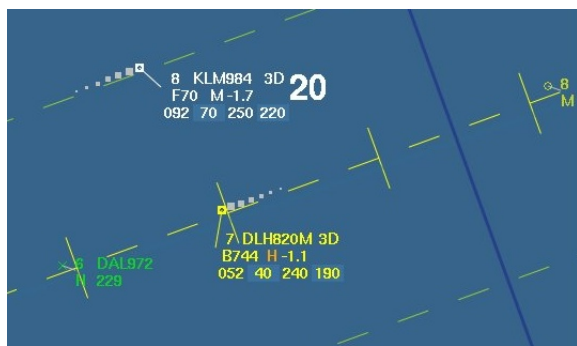
Figure 6. Screenshot of the HMI radar display with the turn-to-base counter at the label of flight “KLM984” (sectional enlargement of Figure 5. ).
