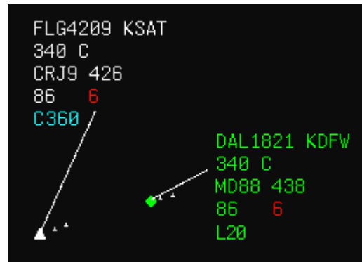
Figure 4. Flight data blocks with conflict notification, resolution advisory and datalink request from aircraft
