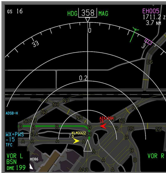
(b) Autonomy level 2 with the additional alerting functions showing conflicts of AL 1 and AL 3.
