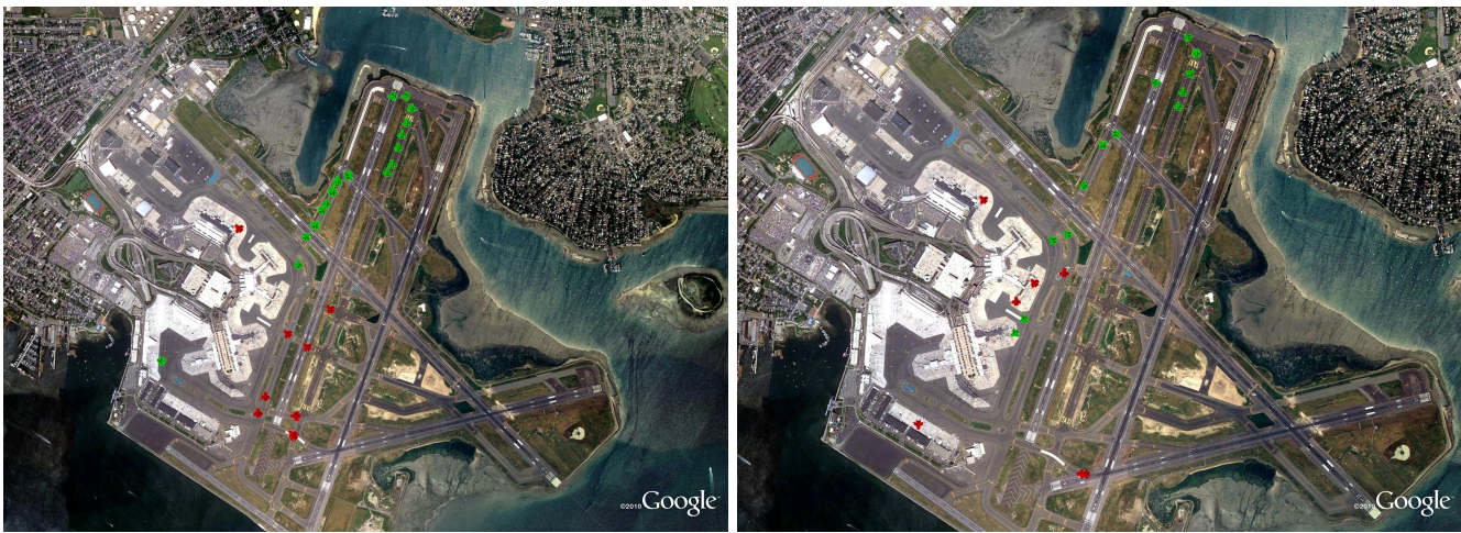
Fig. 10: Snapshots of the airport surface, (left) before metering, and (right) during metering of pushbacks. Departing aircraft are shown in green, and arrivals in red. We note that the line of 15 departures between the ramp area and the departure runway prior to commencement of pushback rate control reduces to 8 departures during metering. The white area on the taxiway near the top of the images indicates the closed portion of taxiway “November”.
