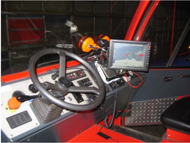
Figure 3. luggage car with integrated onboard unit
