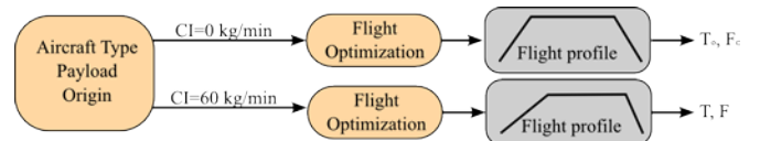
Figure 5: Schema of the flight optimizations performed for each flight in the data set
