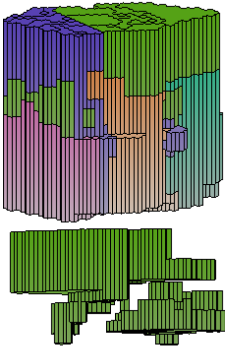
Figure 4. A poor sectorisation by our algorithm, for Munich North ACC, with 4,879 cells of size 10 NM \times 10 NM \times 2000 feet. Top: all five sectors. Bottom: a very awkward sector.
