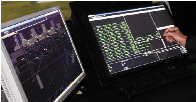
Figure 3: Map (left) and EFS (right) displays for the Ground Controller
