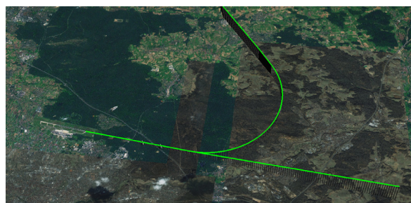
Figure 5. Example RNP AR to Nuremberg, Germany compared to ILS straight-in
