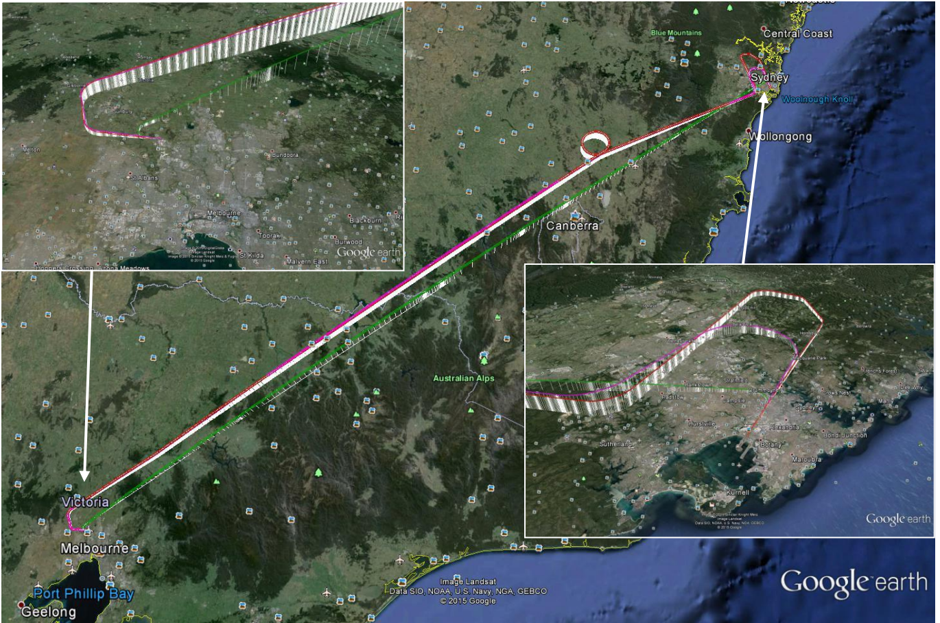
Figure 6. Lateral paths of the Actual Flown Trajectory (red), Procedure-Optimal Trajectory (magenta), and the User Preferred Trajectory (green). The Actual Flown Trajectory experiences one holding pattern and additional vectoring at Sydney resulting in 14% more miles flown over Procedure-Optimal (i.e. flight plan), or 24% over the User Preferred Trajectory. The effect of terminal area procedures is very clear with 8% additional track miles over User Preferred.
