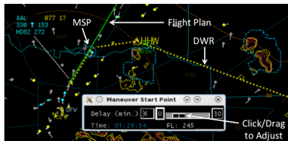
Figure 17. Maneuver Start Point.
