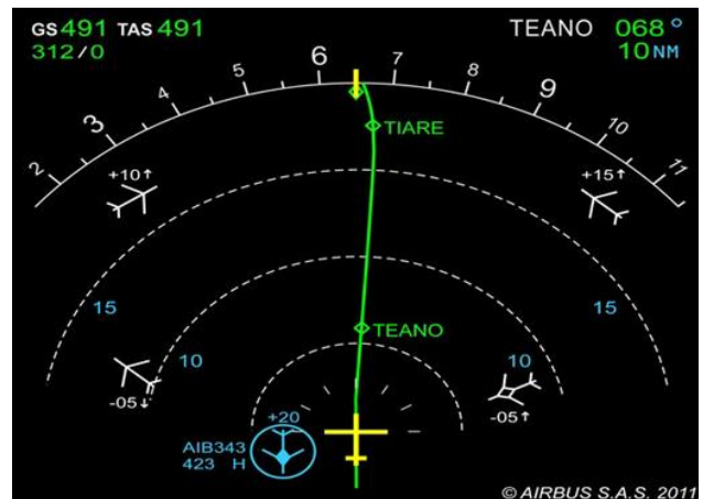
Figure 1. Cockpit Display of Traffic Information by Airbus.
