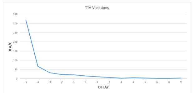
Figure 11. A/C not meeting their TTA with respect to the applied CTOT delay.
