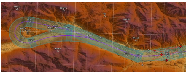
Figure 4. RNP Missed Approach Procedure Protection Area (FPDAM software design by Austro Control)
