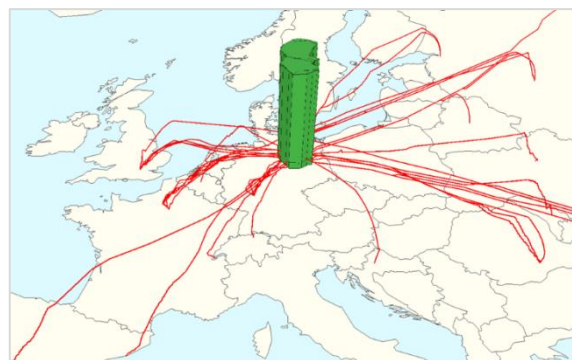
Figure-10 Modelling trajectories through a single control sector in NEST over an hour
