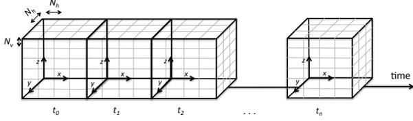
Fig. 8. Four-dimension (3D space + time) grid for conflict detection, illustrated as a time series of 3D grids which is sampled with discretization time step  $\Delta t = t_n - t_{n-1}$ . The size of each cell in the 3D grids is defined by the minimum separation requirements ( $N_h$  and  $N_v$ ).
