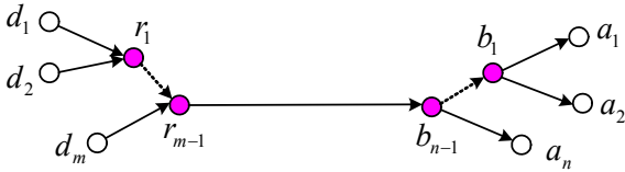
FIGURE 1 WGSMT formation flight path. White circles are origin nodes and pink circles are Steiner nodes.
