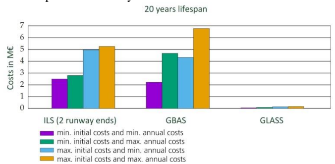
Figure 8 : Comparison of the costs of ILS, GBAS and GLASS over 20 years at a lifespan of the systems of 20 years.
