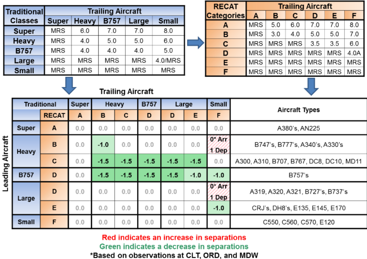
Figure 1. – Change in Separation Requirements (nm)
